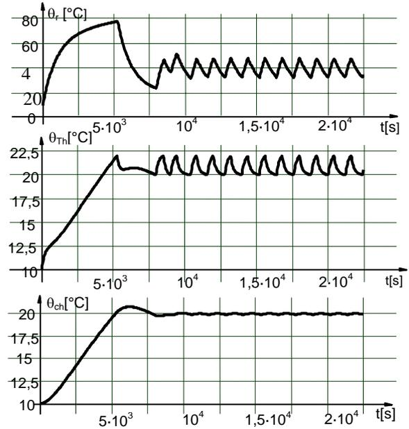
Fig.7 Petri net simulation results for  $c_1 = 10^{-4} \text{ s}^{-1}$ ,  $c_2 = 5 \cdot 10^{-5} \text{ s}^{-1}$ ,  $c_3 = 5 \cdot 10^{-3} \text{ s}^{-1}$ ,  $c_4 = 10^{-3} \text{ s}^{-1}$ ,  $Q_1 = 0.012 \text{ °C/s}$ ,  $Q_2 = 0,06 \text{ °C/s}$ ,  $\theta_{th1} = 20 \text{ °C}$ ,  $\theta_{th2} = 22 \text{ °C}$ ,  $\theta_e = 10 \text{ °C}$ .
