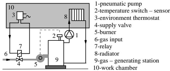
Fig.1 Temperature control process structure
