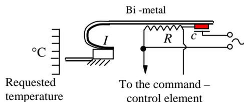
Fig.2 Illustrative for the work principle thermostat
