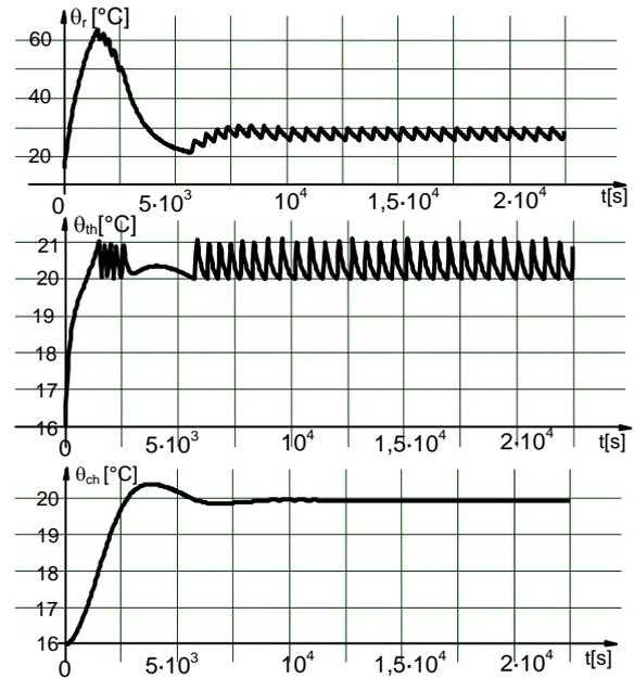
Fig.8 Petri net simulation results for  $c_1 = 10^{-4} \text{ s}^{-1}$ ,  $c_2 = 5 \cdot 10^{-5} \text{ s}^{-1}$ ,  $c_3 = 5 \cdot 10^{-3} \text{ s}^{-1}$ ,  $c_4 = 10^{-3} \text{ s}^{-1}$ ,  $Q_1 = 0.0168 \text{ °C/s}$ ,  $Q_2 = 0,06 \text{ °C/s}$ ,  $\theta_{th1} = 20 \text{ °C}$ ,  $\theta_{th2} = 22 \text{ °C}$ ,  $\theta_e = 16 \text{ °C}$ .
