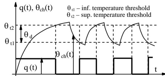
Fig.3 Illustrative to the temperature control process
