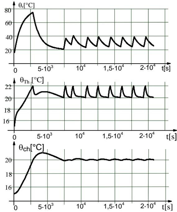
Fig.6 Petri net simulation results for  $c_1 = 10^{-4} \text{ s}^{-1}$ ,  $c_2 = 5 \cdot 10^{-5} \text{ s}^{-1}$ ,  $c_3 = 5 \cdot 10^{-3} \text{ s}^{-1}$ ,  $c_4 = 10^{-3} \text{ s}^{-1}$ ,  $Q_1 = 0.0132 \text{ °C/s}$ ,  $Q_2 = 0,06 \text{ °C/s}$ ,  $\theta_{th1} = 20 \text{ °C}$ ;  $\theta_{th2} = 22 \text{ °C}$ ,  $\theta_e = 15 \text{ °C}$ .
