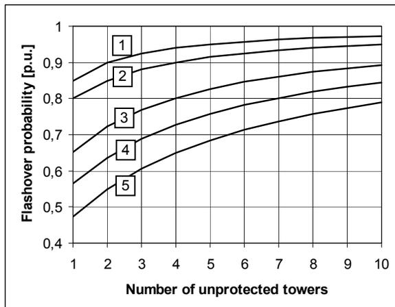
Figure 2: Flashover probability reduction by MOA when the lightning strikes the tower
