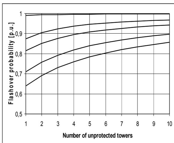
Figure 4: Flashover probability reduction by MOA when the lightning strikes a phase conductor
