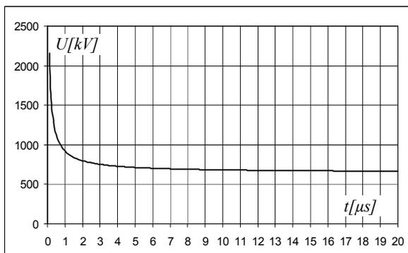
Figure 1: Voltage-time characteristic of the insulator string
