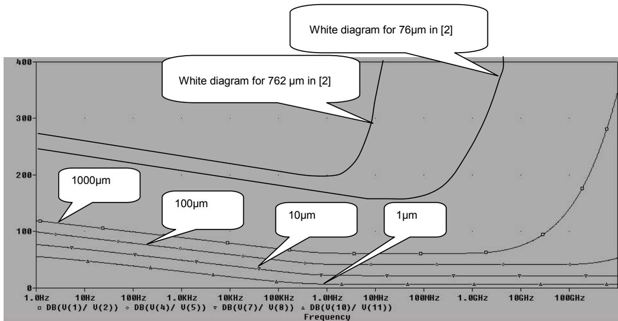
Figure 3: Shielding effectiveness of a copper shield, the highest effectiveness corresponds to the thickest shield
