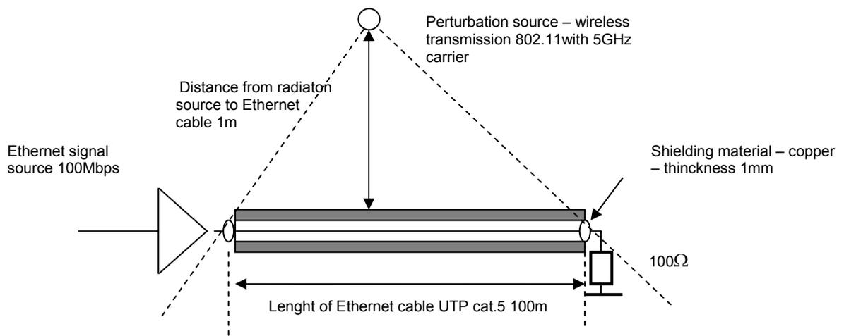
Figure 7: Real configuration for a perturbed Ethernet transmission
