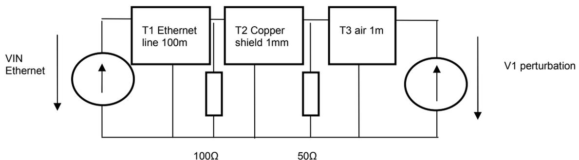
Figure 6: Model and simulation of real configuration for a perturbed Ethernet transmission
