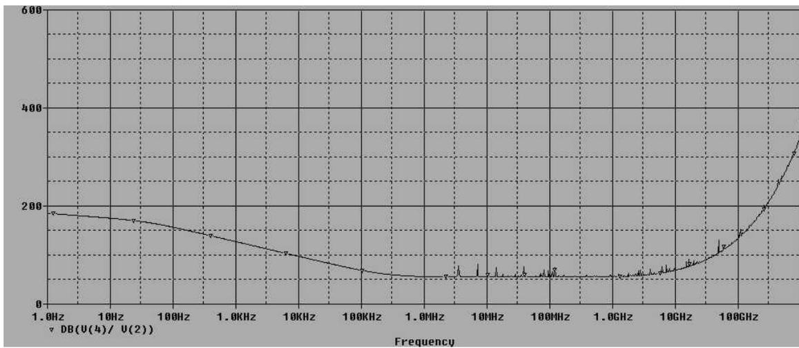
Figure 8: Attenuation introduced by a 1mm copper shield
