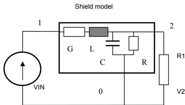
Figure 2: Transmission line model used in modeling a shielding material
