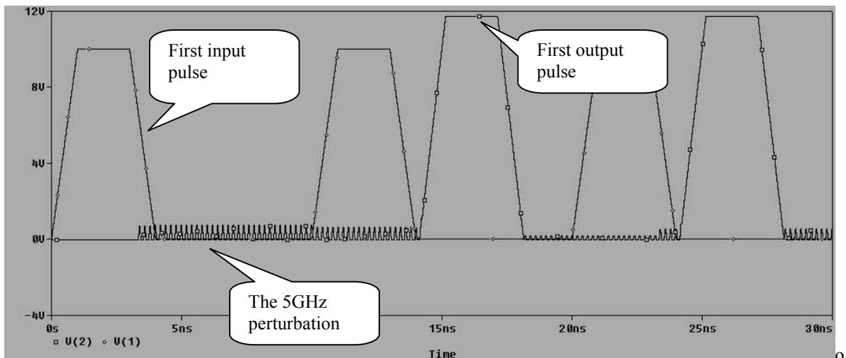
Figure 9: The 5GHz perturbation of the 100MHz Ethernet signal
