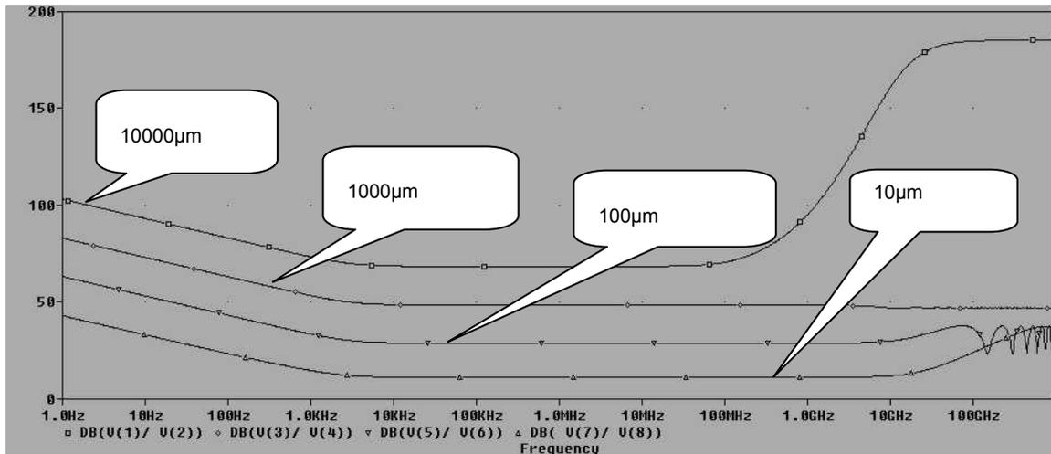
Figure 5: Shielding effectiveness for a nickel shield
