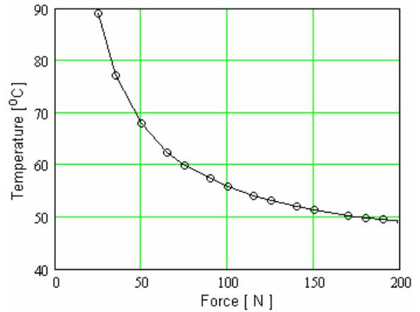
Figure 14: Maximum temperature in contact area versus tightening force (for  $I = 2275 \text{ A}$ )
