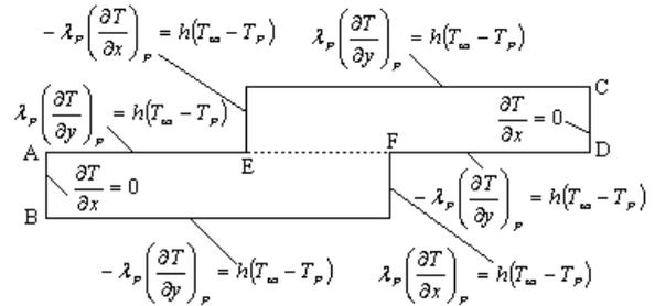
Figure 4: Analysis domain and boundary conditions for thermal model
