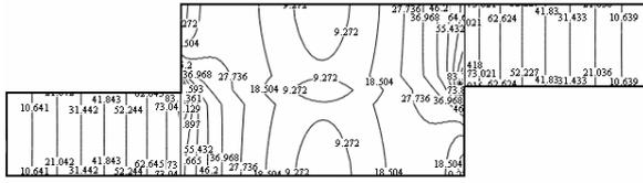
Figure 10: Temperature gradient distribution (in °C/m)
