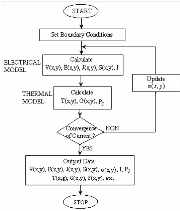
Figure 5: Simplified diagram of numerical algorithm
