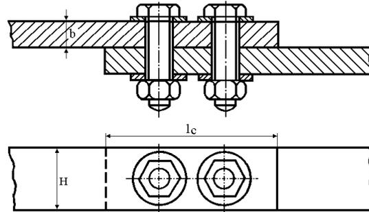
Figure 1: Typical dismantable contacts
