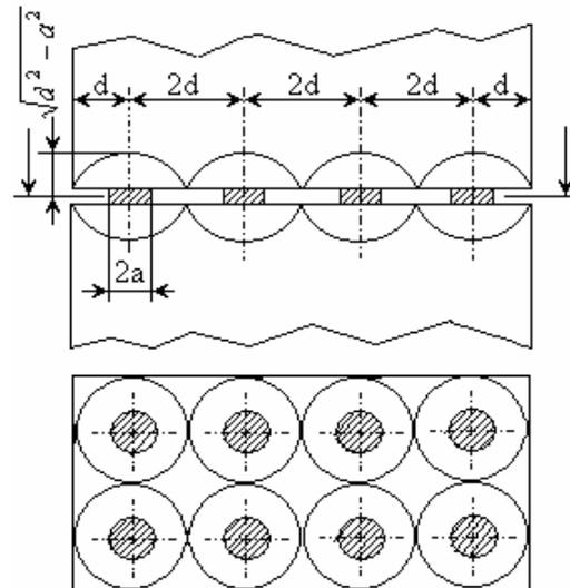
Figure 13: Physical model of contact region
