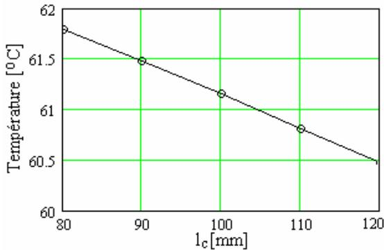
Figure 11: Maximum temperature of contact versus length of contact (for  $S_c = 1.01$  kW).
