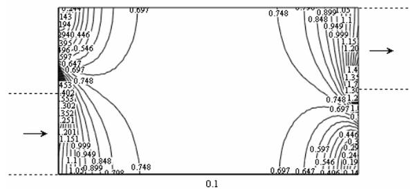
Figure 8: Current density distribution in the contact region (in  $A/mm^2$ )
