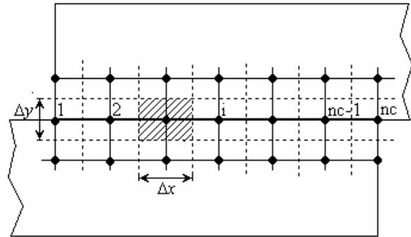
Figure 12: The mesh in contact region
