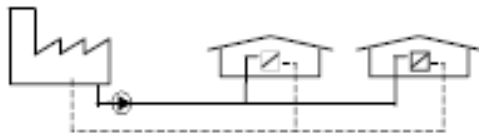
Figure 1: A simple district heating network containing one heat producer and two consumers.
