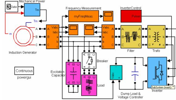
Figure 4: Simulink block diagram of IG-VSI system
