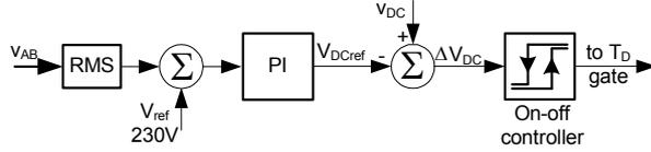
Figure 3: The DC capacitor voltage regulation technique
