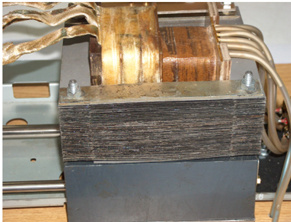
Figure 7: Electric motor with mobile coil in short-circuit.
