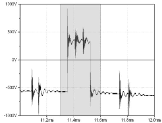
Figure 6: PWM modulated voltage waveform on the motor terminals – low frequency ringing.
