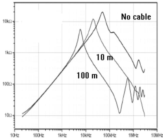
Figure 8: The influence of the converter – motor - cable on the impedance characteristics.
