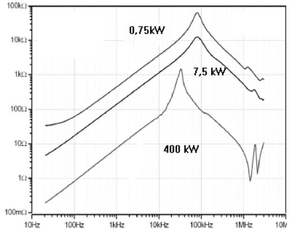
Figure 5: Comparison of the impedance characteristics of the AC motors for different power.
