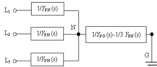
Figure 3: High frequency model of a star connected AC motor.
