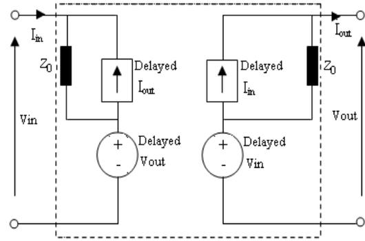
Figure 2: Model of a lossless transmission line.
