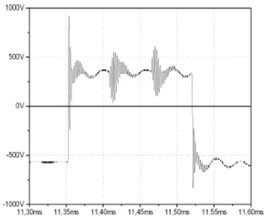
Figure 7: PWM modulated voltage waveform on the motor terminals – high frequency ringing.
