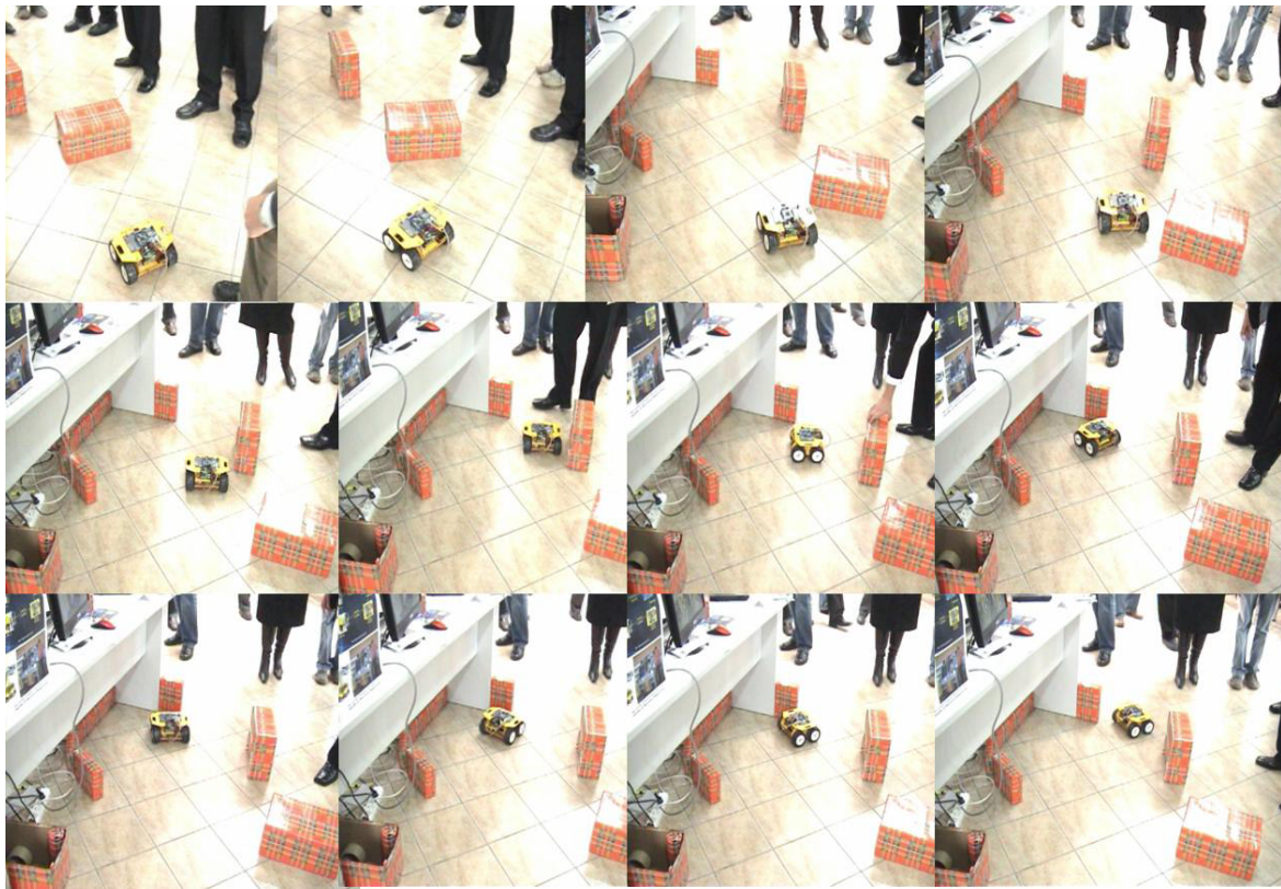
Figure 6. Mobile robot control sequences while avoiding obstacles
