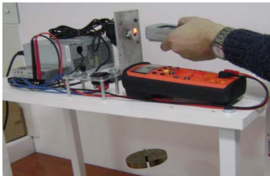
Figure 3: The workbench for measuring the speed in load conditions.
