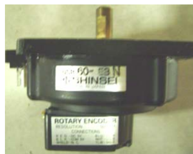
Figure 1: Traveling wave ultrasonic motor. Compact view.
