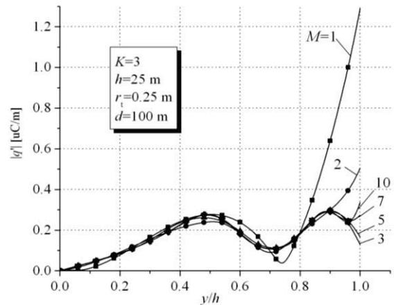
Figure 5: Induced charge distribution along the tower for different tower section numbers.
