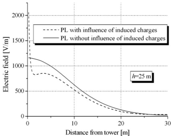
Figure 7: Electric field distribution in vicinity of 2x110 kV power line.
