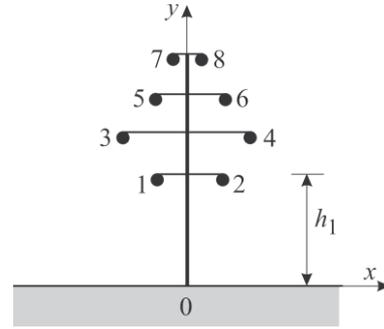
Figure 4: 2x110kV power line cross-section.
