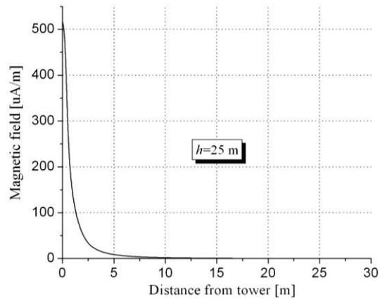
Figure 9: Magnetic field distribution from induced currents on power line tower.
