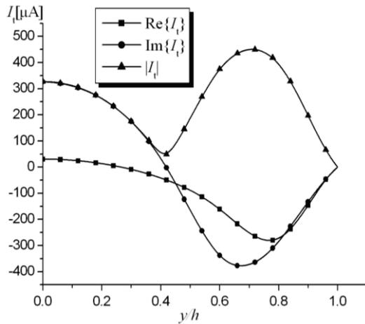
Figure 11: Current distribution along power line tower.
