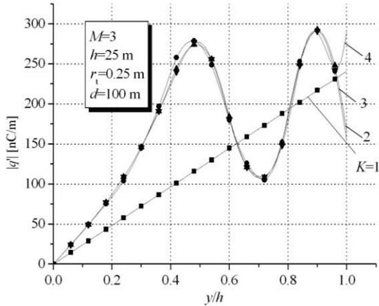
Figure 6: Induced charge distribution along the tower for different polynomial degrees in line charge approximation.
