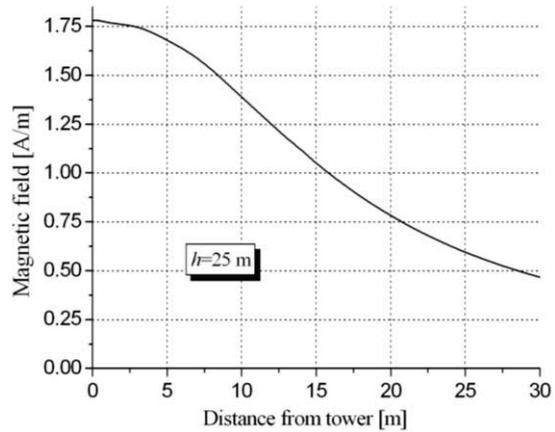
Figure 8: Magnetic field distribution in vicinity of 2x110 kV power line.
