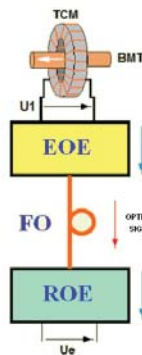
Figure 1: Principle diagram of the hybrid electronic transformer.
