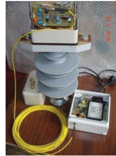
Figure 6: Assembly of the two transformer units optically connected by a 20 m long FO.
