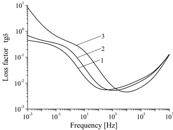
Figure 9: Variation with frequency and temperature of loss factor of oil impregnated paper aged at  $T = 155\text{ °C}$  and  $\tau = 750\text{ h}$  for  $T_m = 30\text{ °C}$  (1),  $50\text{ °C}$  (2),  $90\text{ °C}$  (3).
