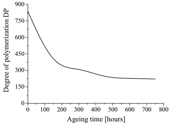
Figure 12: Variation with thermal ageing time of polymerization degree ( $T = 155\text{ }^{\circ}\text{C}$ ,  $\tau = 750\text{ h}$ ).
