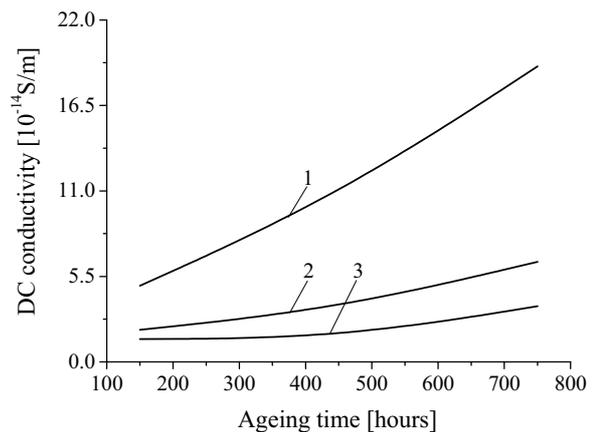
Figure 4: Variation with ageing time  $\tau$  of DC conductivity  $\sigma_{cc}(t)$  of oil impregnated paper at different times  $t$ : 60 s (1), 600 s (2), 3600 s (3) ( $U = 300\text{ V}$ ).
