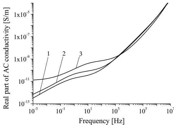
Figure 10: Variation with frequency and temperature of real part of conductivity of oil impregnated paper aged at  $T_m = 155\text{ °C}$  and  $\tau = 750\text{ h}$  for  $T_m = 30\text{ °C}$  (1),  $50\text{ °C}$  (2),  $90\text{ °C}$  (3).
