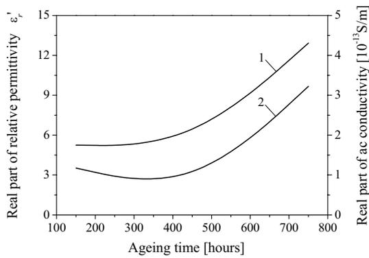
Figure 5: Variation with ageing time  $\tau$  of oil impregnated paper of real part of relative permittivity (1), and electrical conductivity (2) ( $T = 155\text{ }^\circ\text{C}$ ,  $f = 1\text{ mHz}$ ).
