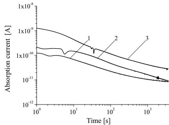
Figure 2: Time variation of absorption currents of oil impregnated paper aged at  $T = 155^\circ\text{C}$  for different times  $\tau$ : 150 h (1), 450 h (2), 750 h (3) ( $U = 300\text{ V}$ ).
