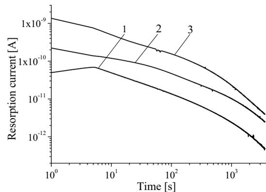
Figure 3: Time variation of resorption currents of oil impregnated paper aged at  $T = 155^\circ\text{C}$  for different times  $\tau$ : 150 h (1), 450 h (2), 750 h (3) ( $U = 300\text{ V}$ ).
