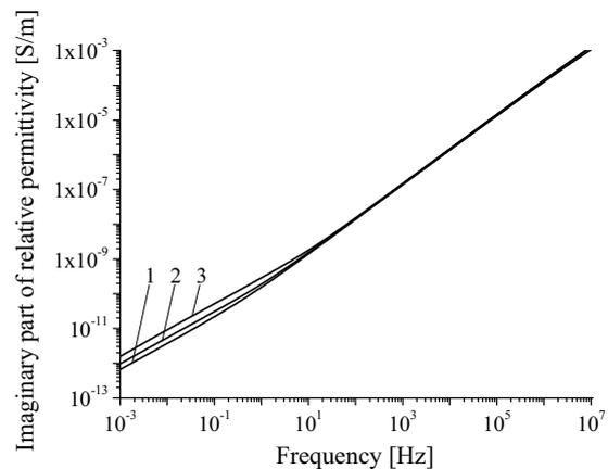
Figure 11: Variation with frequency and temperature of imaginary part of conductivity of oil impregnated paper aged at  $T = 155\text{ °C}$  and  $\tau = 750\text{ h}$  for  $T_m = 30\text{ °C}$  (1),  $50\text{ °C}$  (2),  $90\text{ °C}$  (3).
