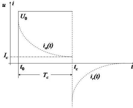
Figure 1: Time variation of absorption ( $i_a$ ) and resorption ( $i_r$ ) currents.
