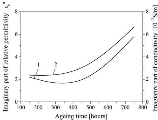
Figure 6: Variation with ageing time  $\tau$  of oil impregnated paper of imaginary part of relative permittivity (1) and electrical conductivity (2) ( $T = 155\text{ }^\circ\text{C}$ ,  $f = 1\text{ mHz}$ ).
