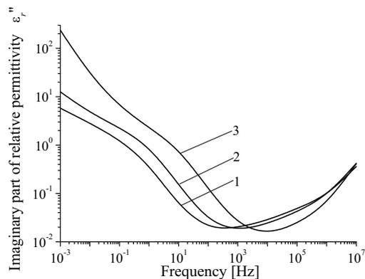
Figure 8: Variation with frequency and temperature of imaginary part of relative permittivity of oil impregnated paper aged at  $T = 155\text{ }^\circ\text{C}$  and  $\tau = 750\text{ h}$  for  $T_m = 30\text{ }^\circ\text{C}$  (1),  $50\text{ }^\circ\text{C}$  (2),  $90\text{ }^\circ\text{C}$  (3).
