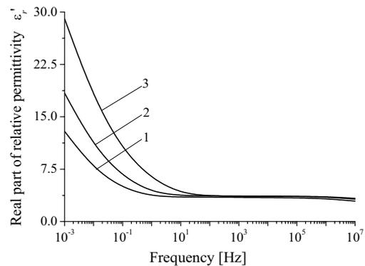
Figure 7: Variation with frequency and temperature of real part of relative permittivity of oil impregnated paper aged at  $T = 155\text{ }^\circ\text{C}$  and  $\tau = 750\text{ h}$  for  $T_m = 30\text{ }^\circ\text{C}$  (1),  $50\text{ }^\circ\text{C}$  (2),  $90\text{ }^\circ\text{C}$  (3).
