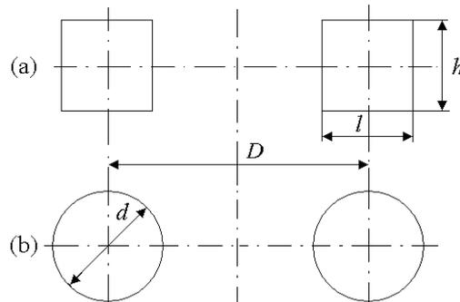
Figure 2: Rectangular cross section toroid (a), circular cross section toroid (b).
