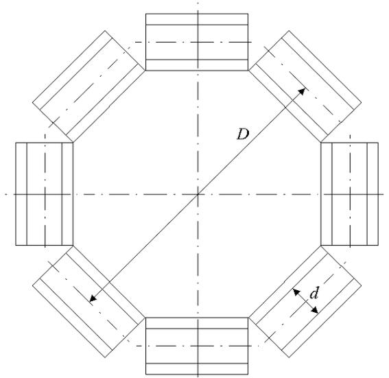
Figure 1: Equatorial cross section of modular toroid.
