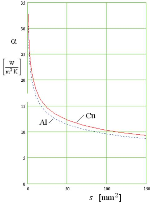
Fig. 4. Heat transfer coefficient versus wire cross section
