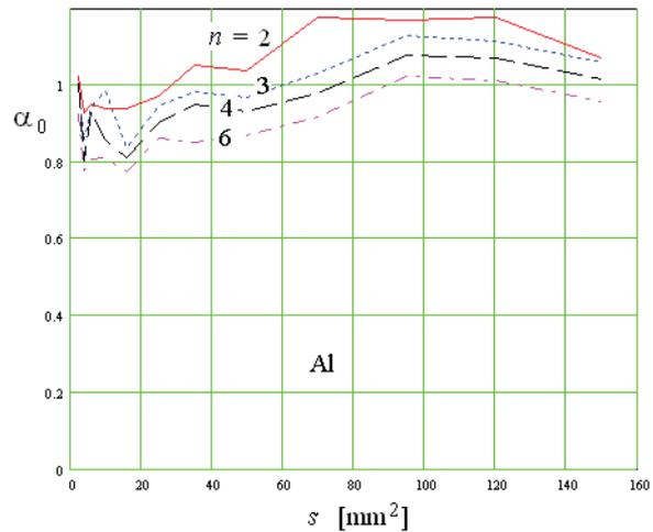
Fig. 3 Values of  $\alpha_0$  determined from the ampacity of Al conductors for 2 up to 5 of them loaded versus wire cross section
