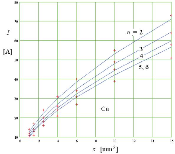
Fig. 5. Ampacities of copper insulating conductors in conduit, calculated with formula (solid line) and I7-2002 (points)
