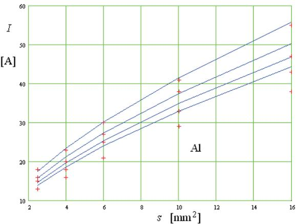
Fig. 6. Ampacities of aluminum insulating conductors in conduit, calculated with formula (solid line) and I7-2002 (points)
