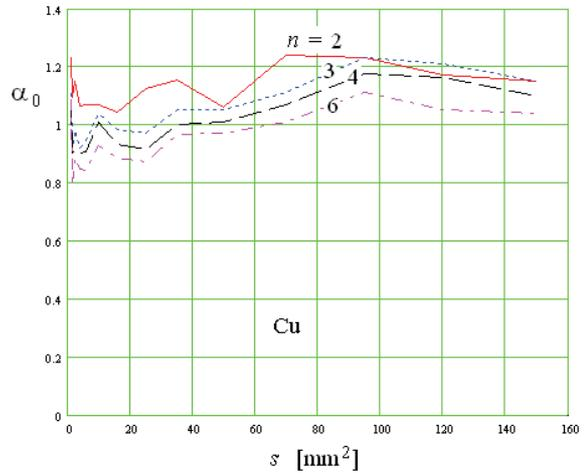
Fig. 2 Values of  $\alpha_0$  determined from the ampacity of copper conductors for 2 up to 5 of them loaded versus wire cross section
