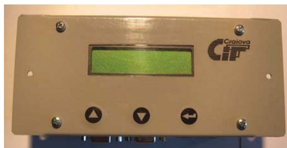
Figure 1: Automaton for monitoring the temperature
