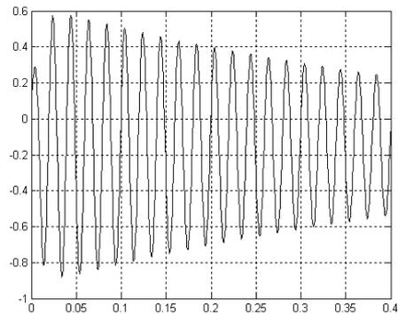
Figure 12: The rotor flux in mobile d-q coordinate system.
