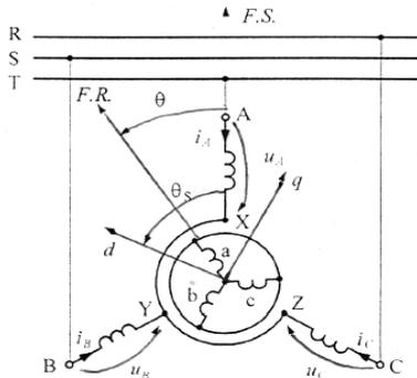
Figure 2: The electrical scheme of an induction motor.
