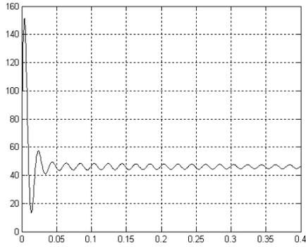
Figure 15: The current  $i_A$  of the first phase.
