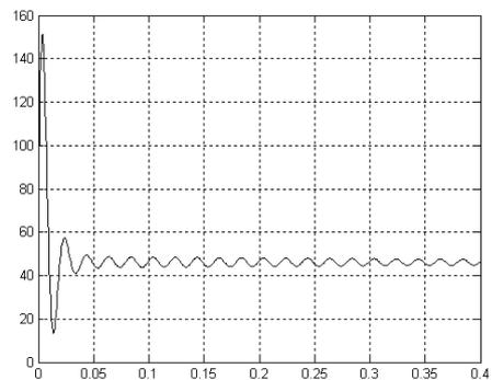
Figure 13: The stator current in mobile d-q coordinate system.
