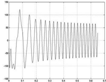
Figure 6: The rotor current in mobile d-q coordinate system.
