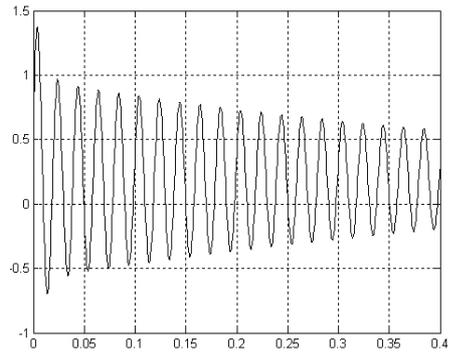
Figure 11: The stator flux in mobile d-q coordinate system.
