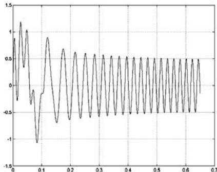
Figure 3: The stator flux in mobile d-q coordinate system
