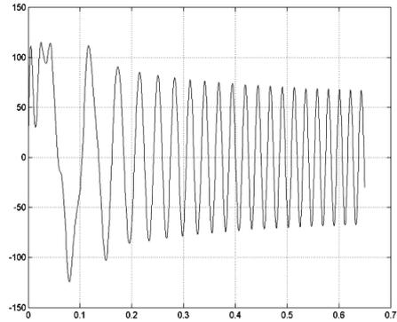
Figure 5: The stator current in mobile d-q coordinate system.
