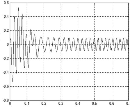
Figure 4: The rotor flux in mobile d-q coordinate system.
