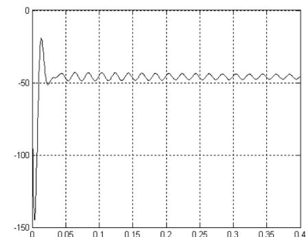
Figure 14: The rotor current in mobile d-q coordinate system.
