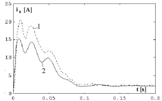
Figure 3:  $i_s$  computed with the help of the experimental values (1) and of the simulated ones (2).
