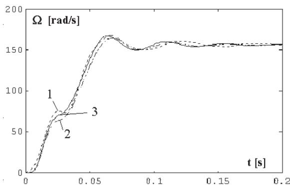
Figure 7: Angular speed determined experimentally (1), by simulating with parameters determined classically (2) and by simulation with parameters resulted by optimization (3).
