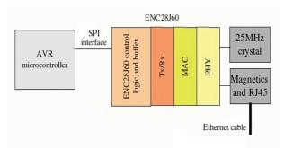
Figure 10. The system's structure
