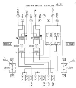
Figure 6: The schematics of connector
