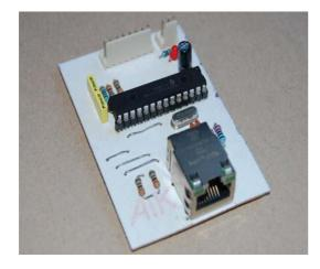
Figure 7: The build of ethernet interface
