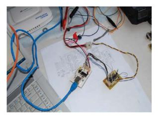
Figure 11. The ethernet interface connected at microcontroller
