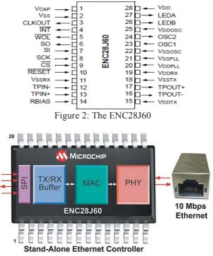
Figure 3. The ENC28J60 block diagram
