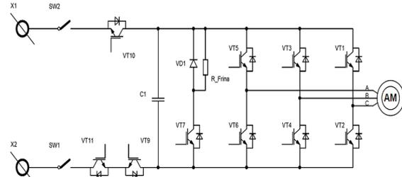
Figure 4. Electric diagram of the power module.
