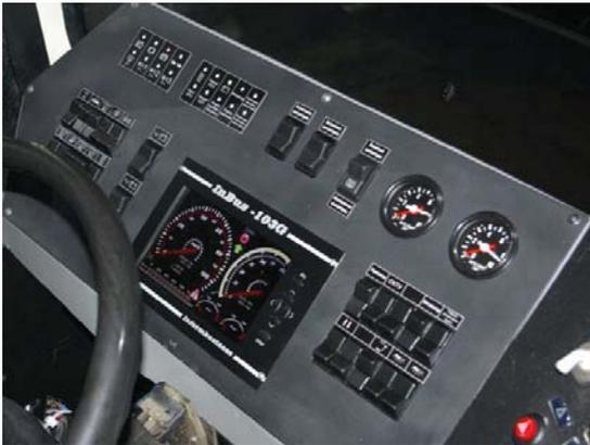
Figure 3. InBus-103G graphic board panel.
