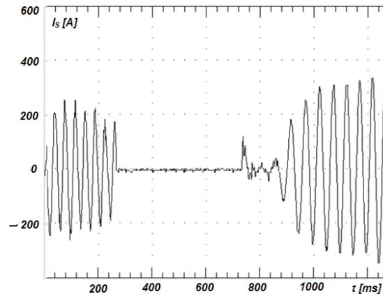
Figure 15. Restarting with residual magnetic flux
