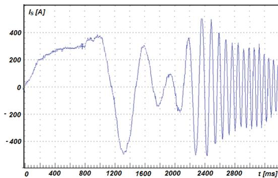
Figure 13. Stator current without compensation block.
