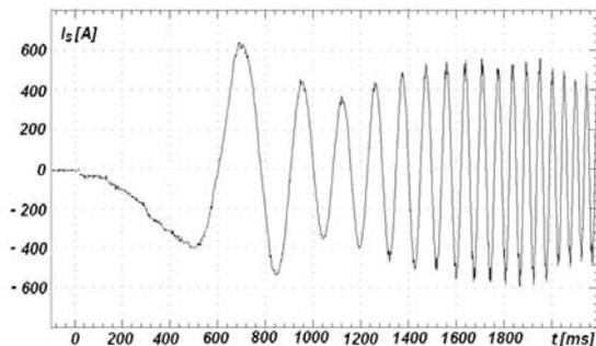
Figure 14. Stator current with compensation block.
