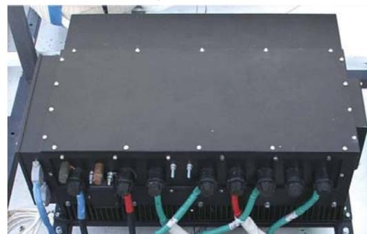
Figure 1. General view of the InBus-103 equipment mounted on the trolley's roof .
