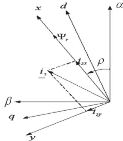
Figure 8 Control vectors in the rotor flux reference frame.
