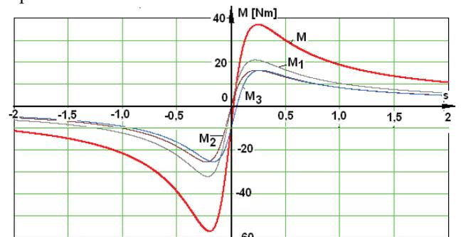
Fig.9. Electromagnetic torques curves appearing in the machine:  $M_1$ ,  $M_2$ , the data voltage and  $U_I$ ,  $U_{II}$ ,  $M_3$  -torque rotor speed relative to  $M$ -torque results.
