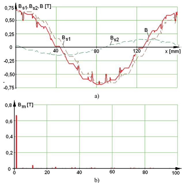
Fig 6. The air-gap flux density curves: a) due to the two sources and the resultant curve; b) harmonic spectrum waveform.
