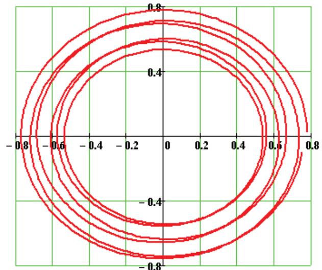
Fig. 15. Phasor locus curve of magnetic induction  $B=f(\omega t)$  for  $\omega t=(0\div 10\cdot 360^\circ)$ .
