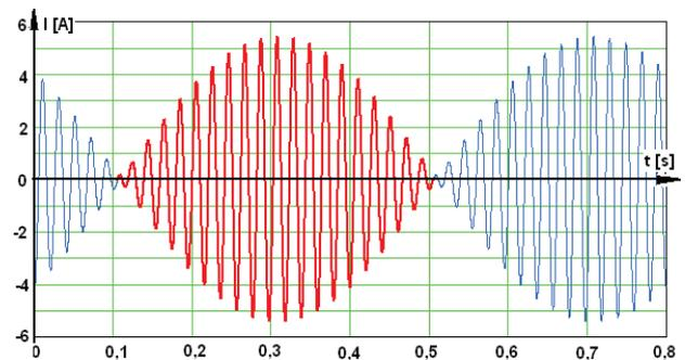
Fig 10. Current curve for the machine functioning with no load.
