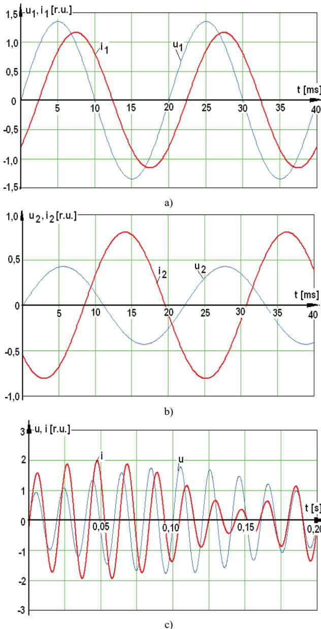
Fig. 4. Voltage and current curves at no load regime: a) at the terminal of  $GS_I$  source ; b) at the terminal of  $GS_{II}$  source; c) at terminal motor for one period.
