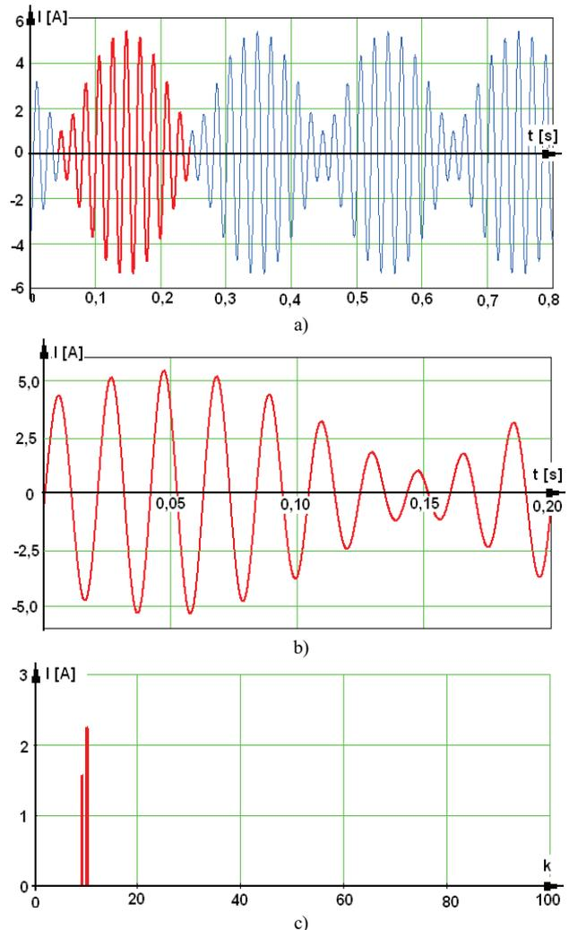
Fig. 5. Current curve at no load regime: a) at motor terminals; b) for a period; c) harmonic spectrum.
