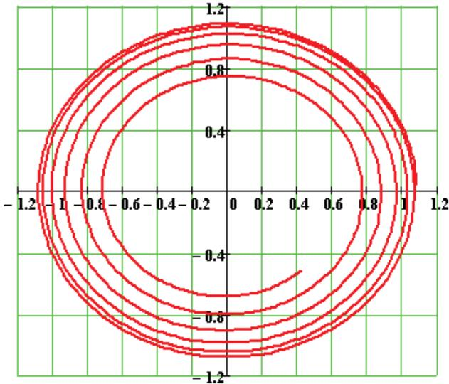
Fig. 11. Phasor locus curve of magnetic induction  $B=f(\omega t)$  for  $\omega t=(0\div 10\cdot 360^\circ)$ .
