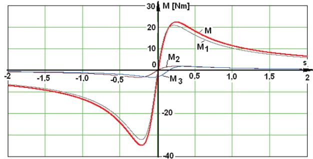
Fig. 13. Electromagnetic torques curves appearing in machine:  $M_1$ ,  $M_2$  – resulting on voltages  $U_I$ ,  $U_{II}$ , and  $M_3$  – the torque relative to rotor speed,  $M$ –resultant torque.
