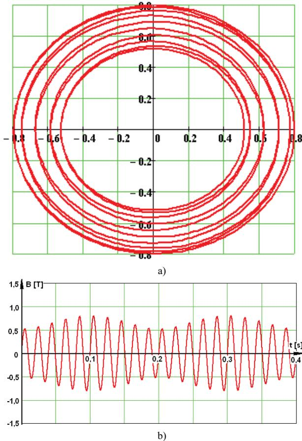
Fig.7. Phasor locus curve of magnetic induction  $B=f(\omega t)$ : a) for  $\omega t=(0 \div 10 \cdot 360^\circ)$ ; b) detail.
