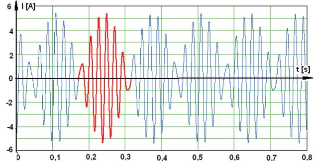
Fig. 14. Current curve- for no load regime of the machine.
