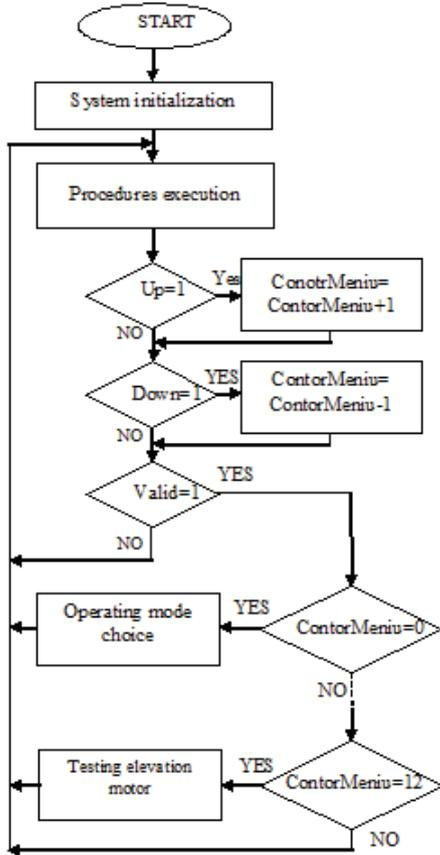
Fig. 9. Flowchart of microcontroller program
