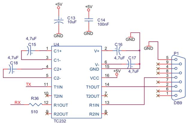
Fig. 5. Electronic circuit of the control TTL module - RS232 interface
