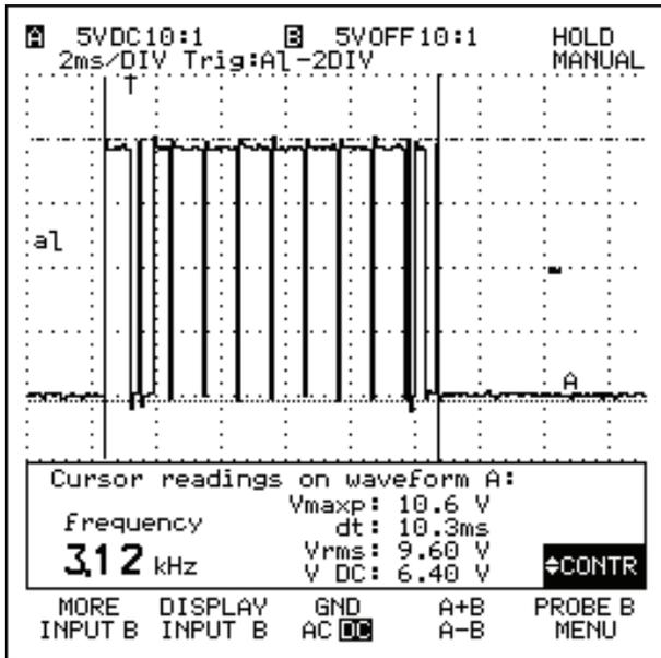
Fig. 15. Sending of a data packet to PC
