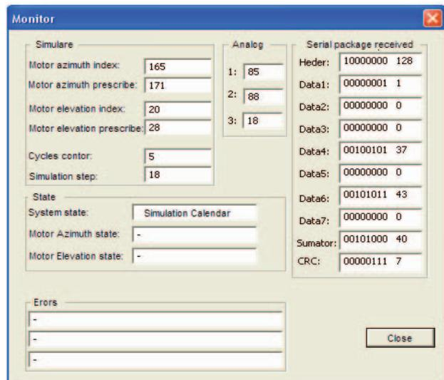
Fig. 14. “Monitor” Window – stepper motors are enabled
