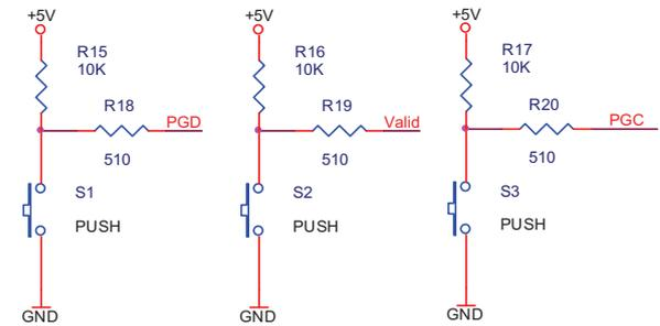
Fig. 4. Electronic circuit of the control module – keyboard block
