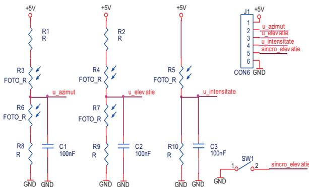
Fig. 7. Electronic circuit of the illumination sensors
