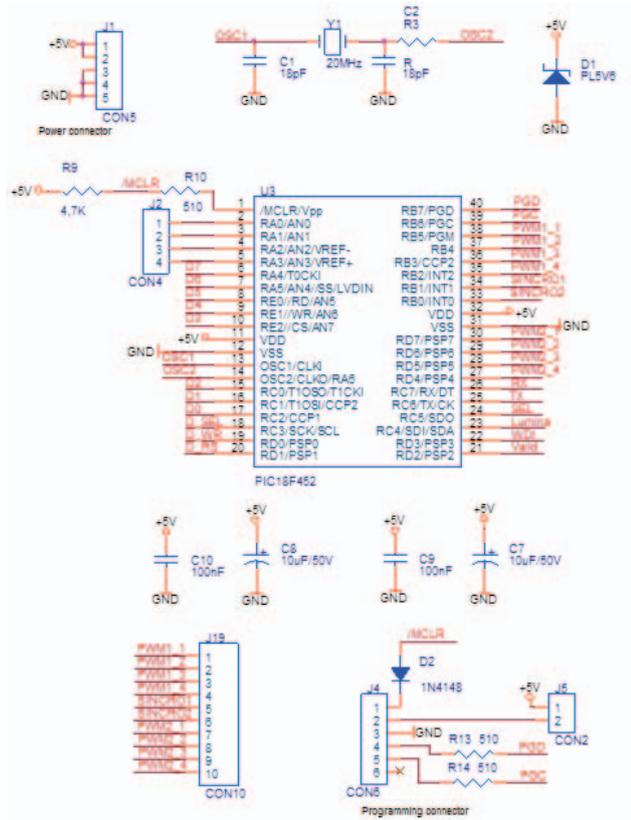
Fig. 2. Electronic circuit of the control module - microcontroller block
