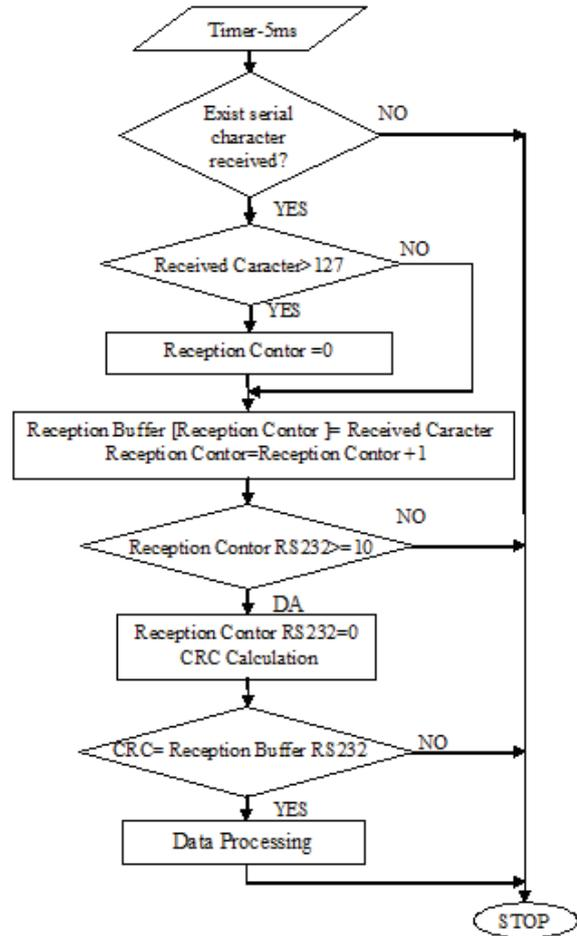
Fig. 10. Flowchart of PC communication procedure
