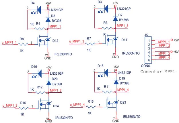
Fig. 6. Electronic circuit of the amplifier block 1- azimuth motor
