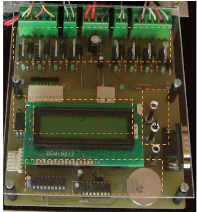
Fig. 8. Final hardware board of automaton: 1- amplifier circuit; 2- micro-controller; 3- display; 4 – keyboard; 5- RTC circuit
