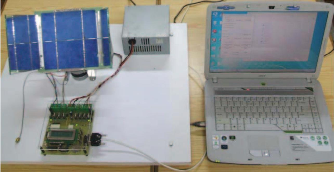
Fig. 12. Experimental model of tracking system for LCPV panel
