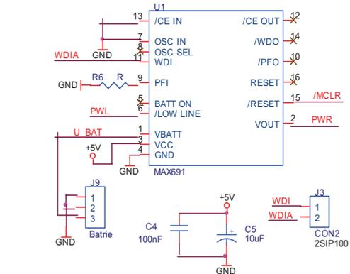
Fig. 3. Electronic circuit of the control module – real time clock block
