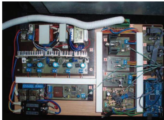
Fig. 3. The control board with microcontroller Arduino Mega 2560
