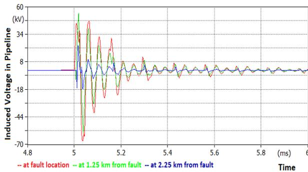
Fig. 13. Induced voltage waveforms in the underground pipeline in case of lightning strike to the upper phase wire.
