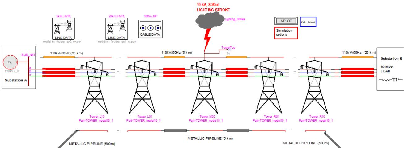
Fig. 2. Part of the EMTP\_RV Model of the analyzed system.
