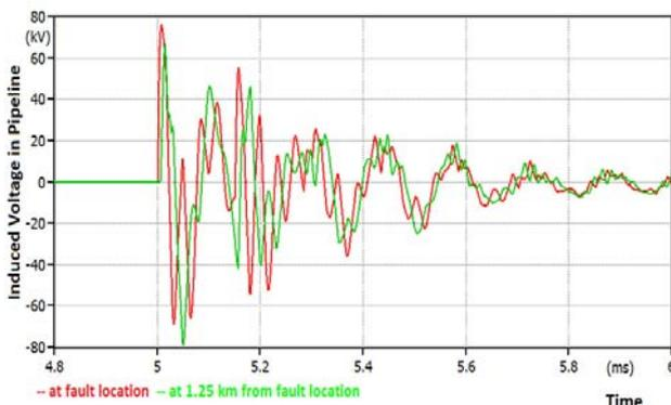
Fig. 14. Induced voltage waveforms in the presence of a mitigation wire for the case of the lightning strike to sky wire with back flashover.
