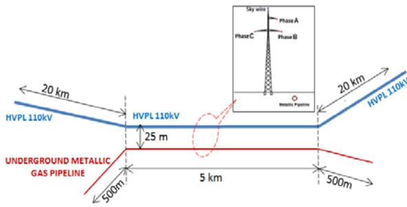
Fig. 1. Over view of the investigated right-of-way
