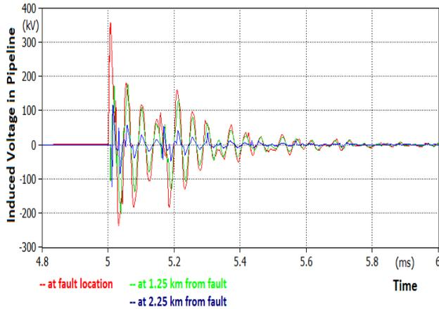
Fig. 9. Induced voltage waveforms in case of lightning stroke to sky wire with back flashover phenomena.
