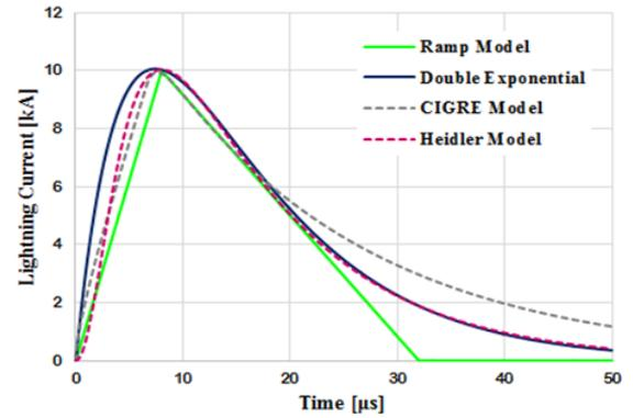
Fig. 4. 10 kA, 8/20  $\mu$ s lightning current implementation with different mathematical functions.
