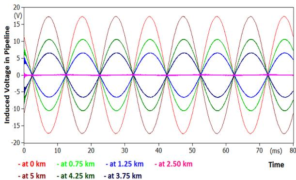
Fig. 6. Induced voltage waveform at different location along the common HVPL-MP right of way.
