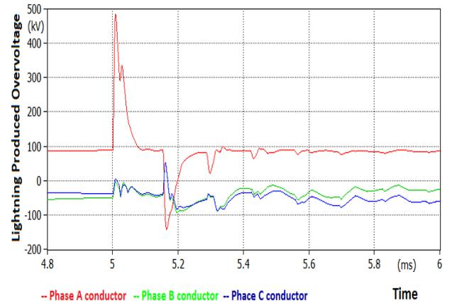
Fig. 12. Induced voltage waveforms in the underground pipeline in case of lightning strike to the upper phase wire.
