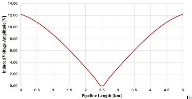
Fig. 5. Induced voltage along pipeline length.
