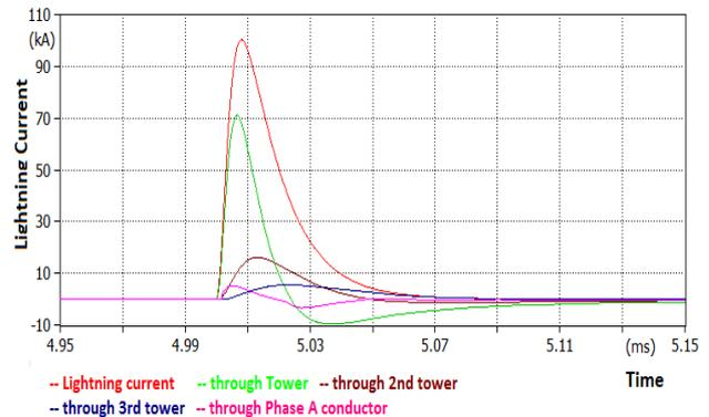
Fig. 7. Produced fault current due to lightning stroke.
