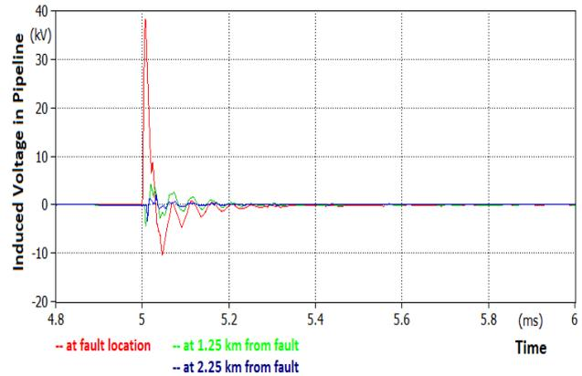
Fig. 11. Induced voltage waveforms in case of lightning stroke to sky wire with no back flashover phenomena triggered.
