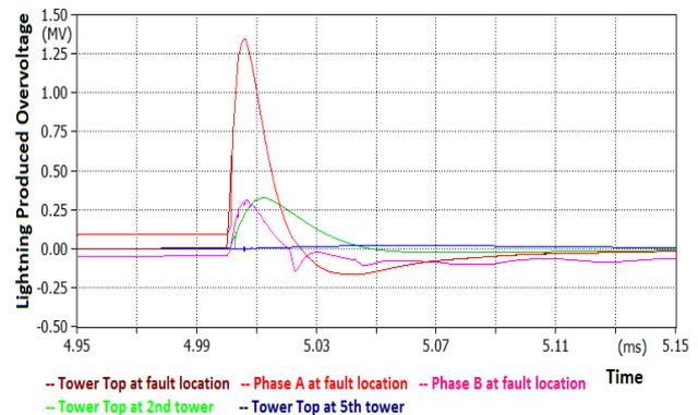
Fig. 8. Produced overvoltage waveforms on power line towers.
