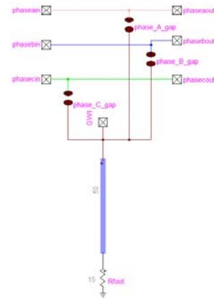
Fig. 3. Model circuit of the 110kV tower
