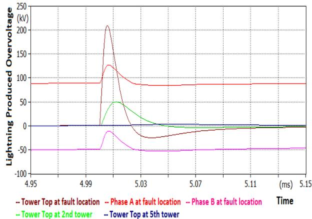
Fig. 10. Produced overvoltage waveforms on power line towers in case of lightning stroke to sky wire with no back flashover triggered.
