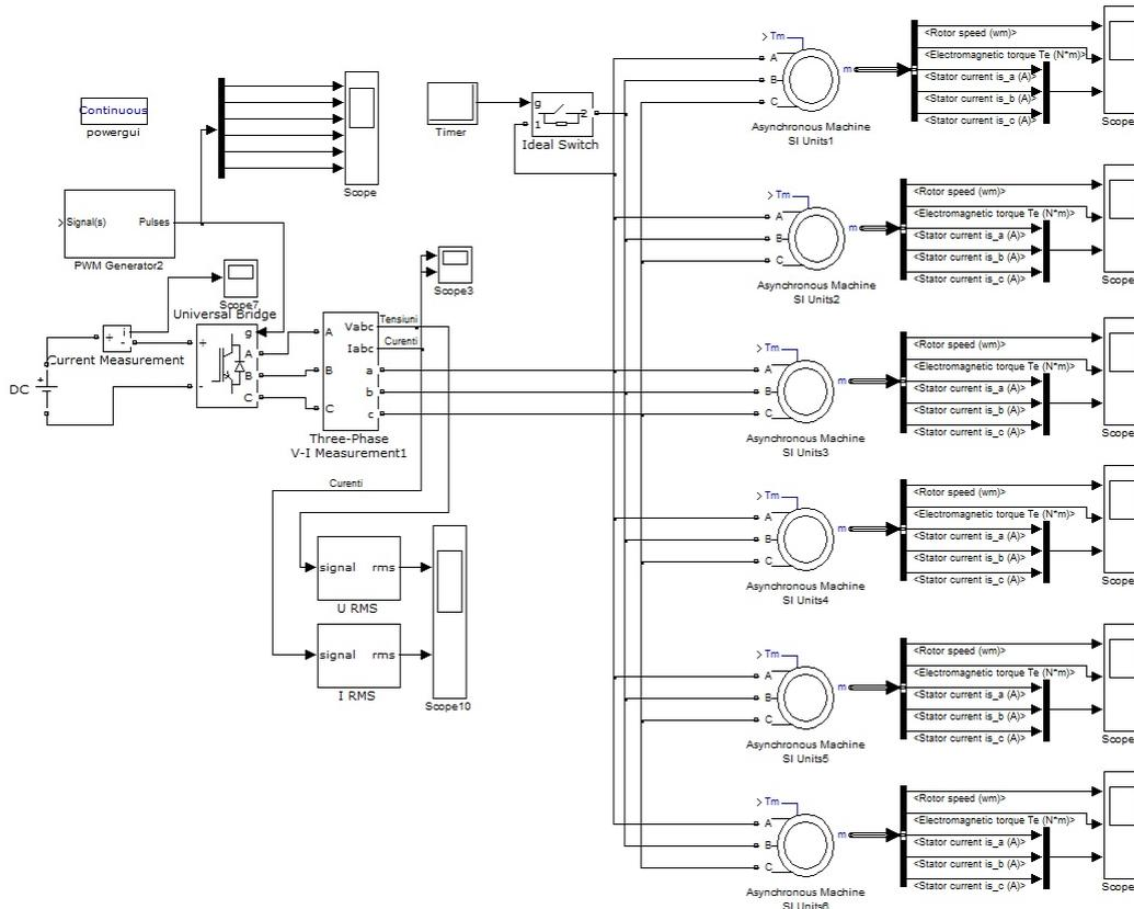
Fig. 14. The Simulink model for “biphasic shortcircuit at inverter output” fault
