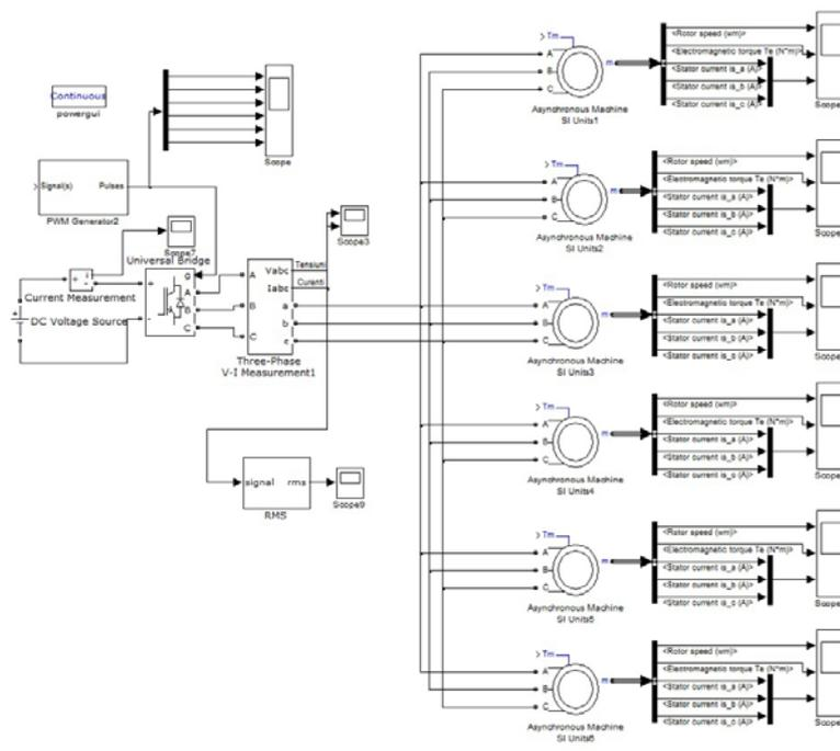
Fig. 1. The Simulink model of the auxiliary ventilation services.
