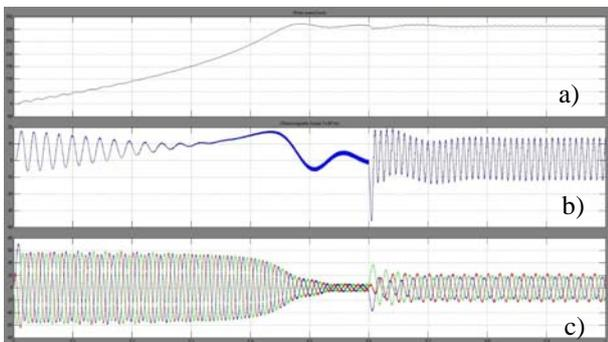
Fig. 15 – The waveforms of motor speed (a), electromagnetic torque (b) and currents (c) in the fault regime
