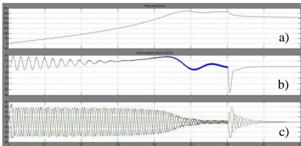
Fig. 8 The speed (a), electromagnetic torque (b) and the stator currents (c) vs. time after the appearance of defect
