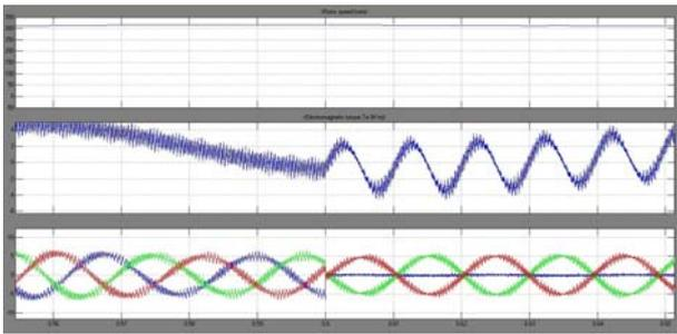
Fig. 13. The speed, electromagnetic torque and motor currents - itemized
