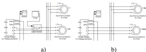
Fig. 9. The difference between the original model (b) and the model simulated fault (a)
