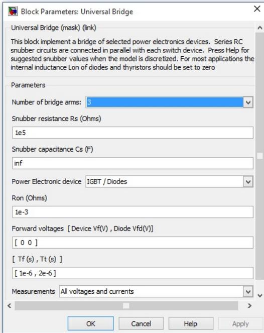
Fig. 3. The inverter block
