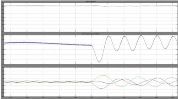
Fig.16. –The waveforms of motor speed, electromagnetic torque and currents - fault regime, itemized
