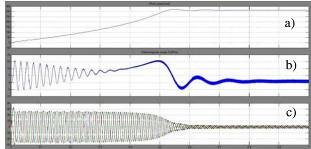
Fig. 5. The rotation speed (a), electromagnetic torque (b) and the currents (c) vs. time for a motor
