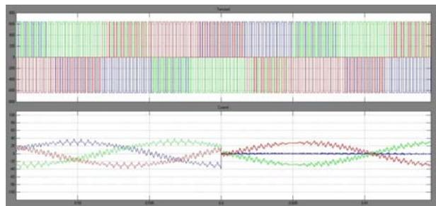
Fig. 11. Instantaneous values of voltages and currents at the inverter output - itemized
