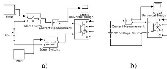
Fig. 6. The difference between the original model (b) and the model of the simulated fault (a)
