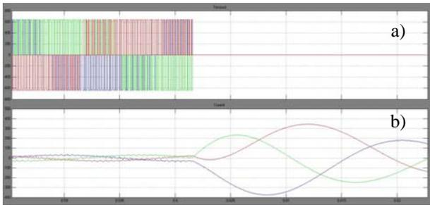
Fig. 7. The instantaneous values of voltages (a) and currents (b) vs. time at the inverter output
