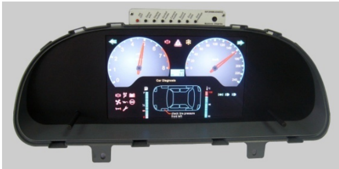
Fig. 10. Experimental on-board panel based on Fujitsu "Lime" MB86276.
