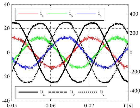
Fig. 11 The current absorbed from the power grid in traction operation when the desired grid current computation is based on the distorted load current
