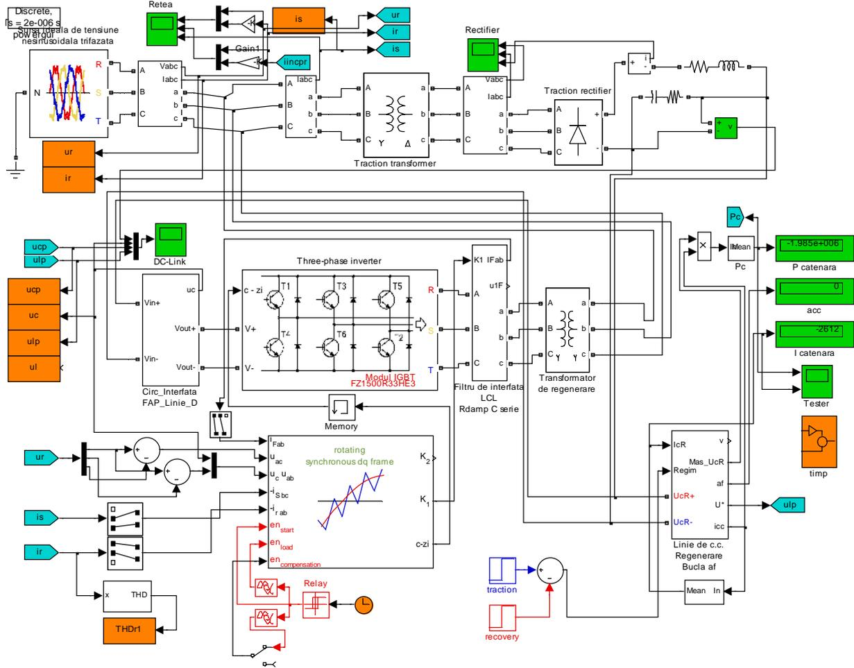
Fig. 3. The Simulink model of the active urban traction dc substation
