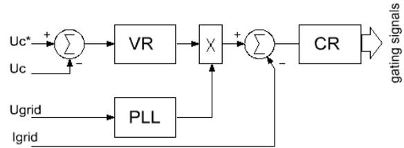
Fig. 2. The active compensator control algorithm based on the DC-Link voltage controller
