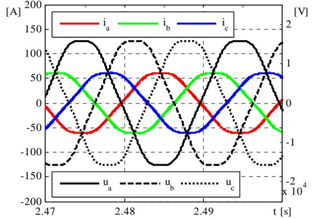
Fig. 6. The current generated to the power grid in recovery operation when the desired grid current computation is based on the distorted load current
