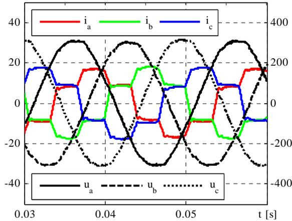
Fig. 10. The current absorbed from the power grid by the experimental rectifier
