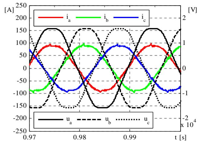
Fig. 7. The current absorbed from the power grid in traction operation when the desired grid current computation is based on the DC-Link voltage controller
