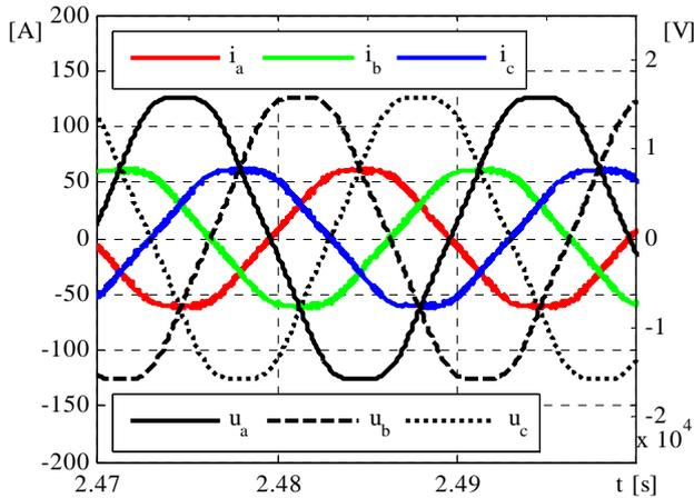
Fig. 8. The current generated to the power grid in recovery operation when the desired grid current computation is based on the DC-Link voltage controller
