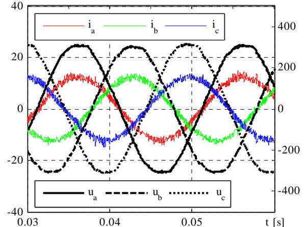
Fig. 12. The current absorbed from the power grid in traction operation when the desired grid current computation is based on the DC-Link voltage controller
