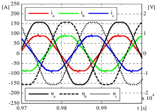
Fig. 5. The current absorbed from the power grid in traction operation when the desired grid current computation is based on the distorted load current
