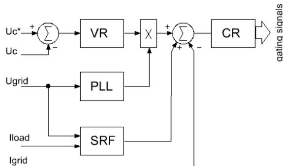
Fig. 1. The active compensator control algorithm based on the distorted load current
