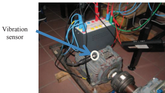
Fig. 16. Measurement of SPMSM vibrations in faulty case.
