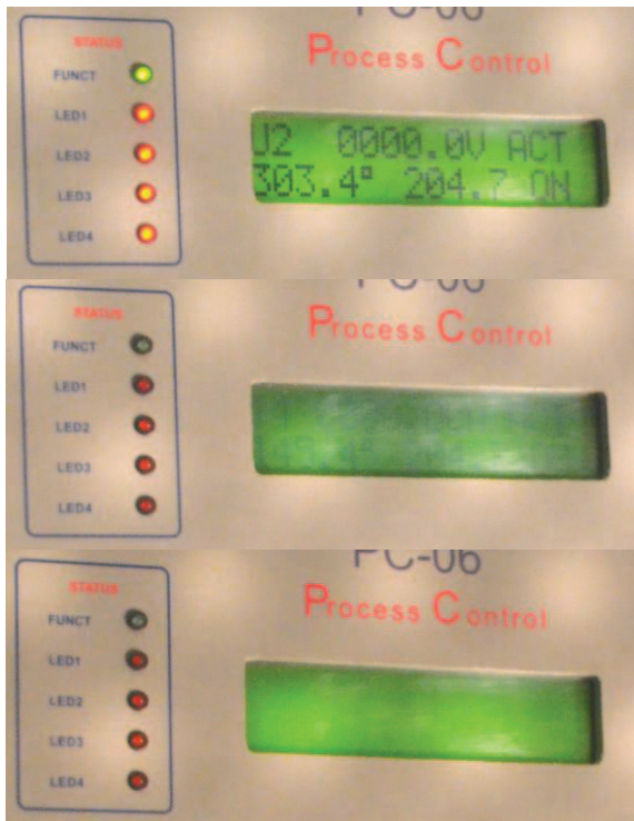
Fig. 10. DAS behavior at resetting for 451 MHz.
