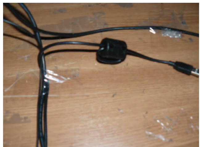
Fig.3 Ferrite installed on USB cable
