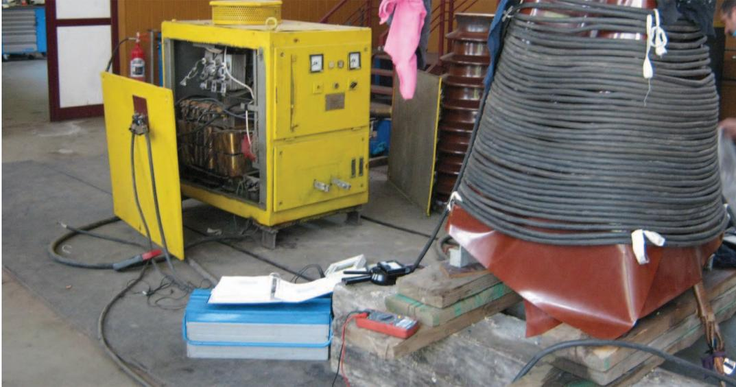
Fig. 1. Detail about the drying of current transformers in actual technology.
