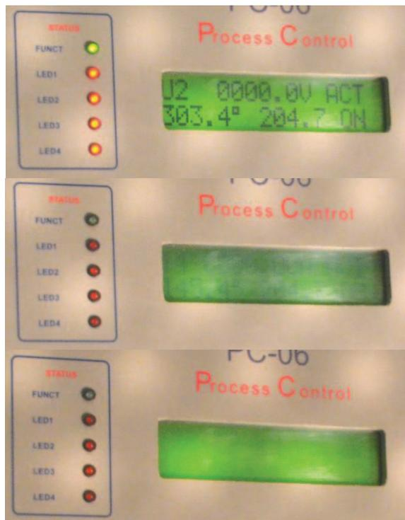
Fig. 10. DAS behavior at resetting for 451 MHz.
