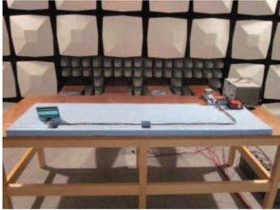
Fig. 8. Setup for the determination of disturbances transmitted through radiation for EUT
