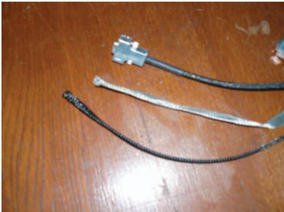
Fig.5 VGA shielded cable
