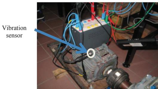
Fig. 16. Measurement of SPMSM vibrations in faulty case.
