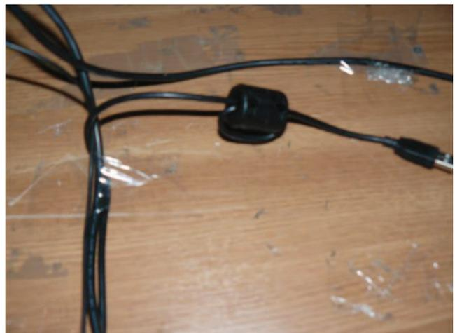
Fig.3 Ferrite installed on USB cable
