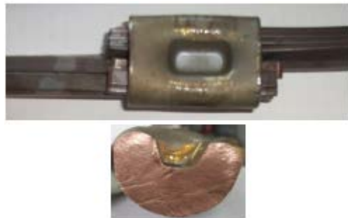
Fig. 1. Crimped connection sample used for analyzes.
