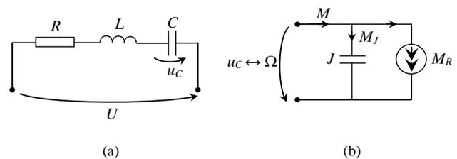
Fig. 3.  $RLC$  series circuit (a) and the complementary equivalent electrical diagram for the motion equation (b).
