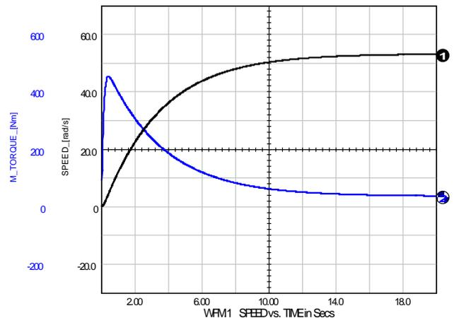
Fig. 6. The time variations of the angular speed (1) and of the motor torque (2) during the starting, obtained in SPICE.
