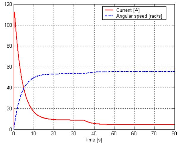
Fig. 2. Time variations of the current and of the angular speed during starting and torque variation (analytical method).
