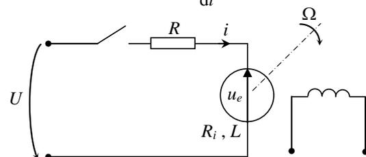
Fig. 1. Schematic circuit of a separately excited direct current machine.
