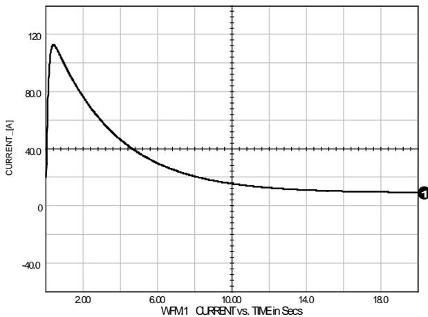
Fig. 5. The time variation of the armature current during the starting, obtained in SPICE.
