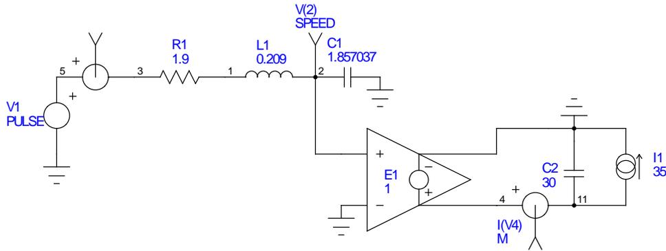
Fig. 4. RLC series circuit and motion equation implemented in SPICE.
