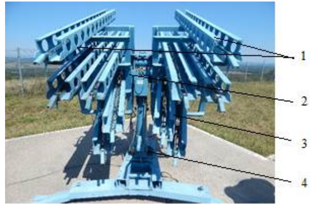
Fig.13. Mechanical structure of a launch pad: 1- launch girder; 2- shelf; 3- distribution block; 4- azimuth/elevation cradle.
