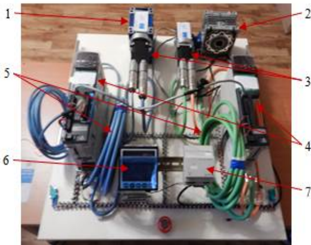
Fig.15. An experimental model of positioning system: 1- mechanical gear for elevation; 2- mechanical gear for azimuth; 3- synchronous motors; 4 – smart drivers; 5- communication cables; 6 – touchscreen; 7- DC power supply.
