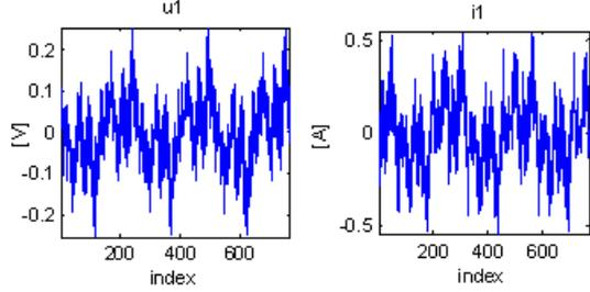
Fig. 3. Waveforms representing reconstruction errors when using DWT and 'db20r'.
