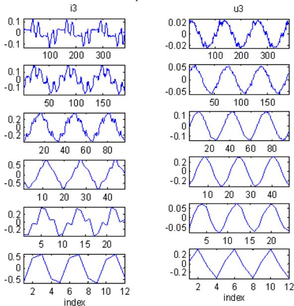
Fig. 13. Differences between the vectors of details generated with ‘db14’ and ‘db14r’. Levels increasing from top to down.
