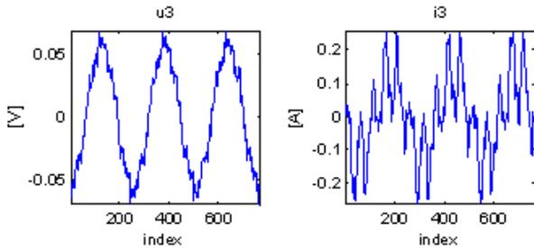
Fig. 4. Waveforms representing reconstruction errors when using SWT and 'db20r'.
