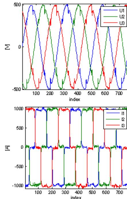
Fig. 1. Acquired waveforms (interpolated with spline). Top - currents; bottom - Voltages.
