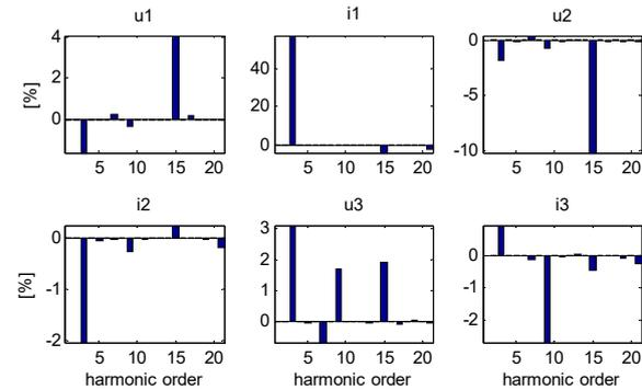
Fig. 6. Percent relative errors for harmonic spectra, considering 'db14r' relative to 'db14'.
