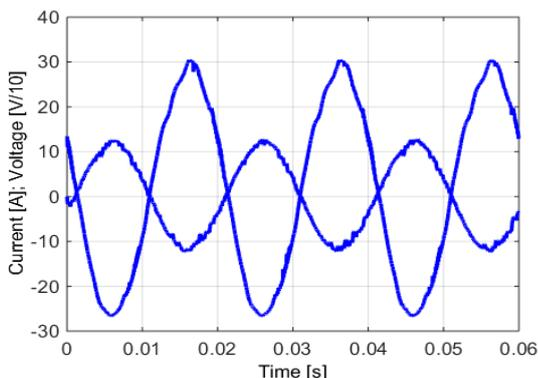
Fig. 11. The grid phase voltage and current in recovery regime.
