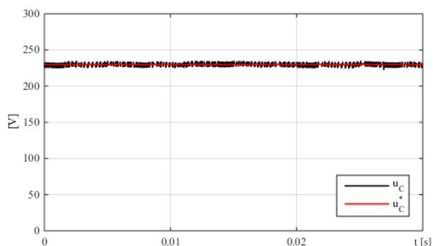
Fig. 5. Detail of evolution of the voltage across the compensation capacitor during the filtration regime.
