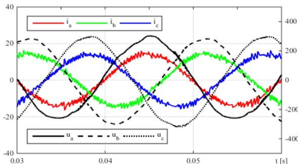
Fig. 6. The grid phase voltages and currents in traction/active filtering regime.
