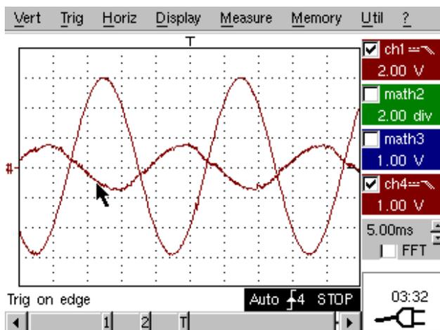
Fig. 12. The grid line voltage and current in recovery regime recorded by oscilloscope.
