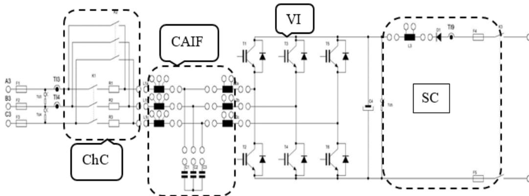
Fig. 1. Electric scheme of the power part of experimental model of SISFREG.
