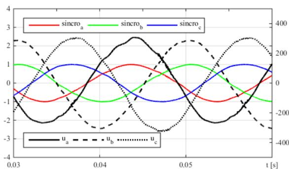
Fig. 9. The grid phase voltages and their templates obtained by PLL loop.
