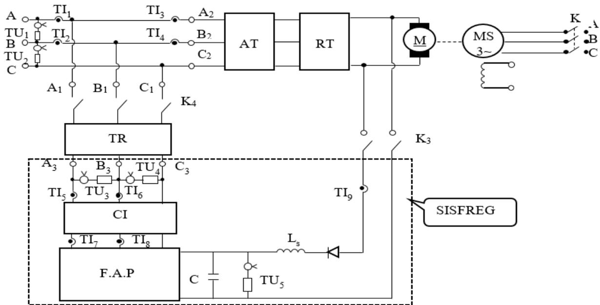
Fig. 2. Electric scheme of the experimental testing stand.
