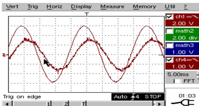
Fig. 7. The grid line voltage and current in traction/active filtering regime.
