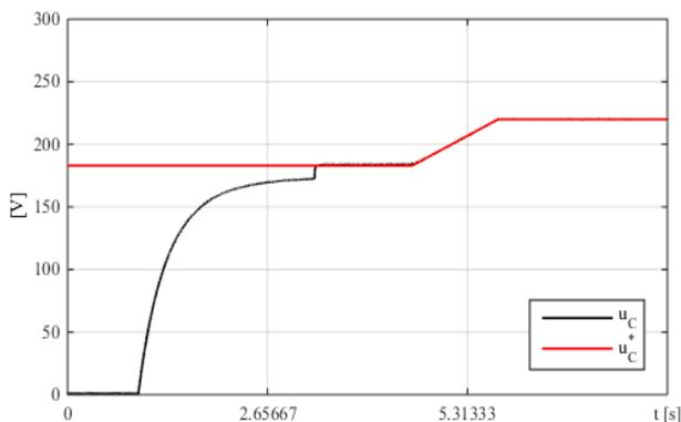
Fig. 4. Evolution of the voltage across the compensation capacitor during the charging process (prescribed-red; real-black).
