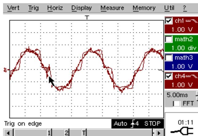
Fig. 14. The load and the grid currents for L1=0.8 mH.
