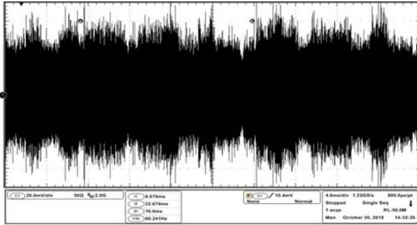
Fig. 8. Video signal - two thick horizontal bars and a thin one, using a LISN and a shielded power supply
