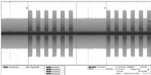
Fig. 5. Video signal - 6 horizontal lines, using MDS-21 clamp and a shielded power cable
