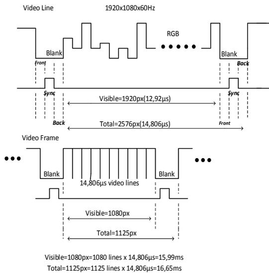
Fig. 1. The structure of an analogical video signal for the 1920 x 1080 resolution at 60 (Hz) refresh rate
