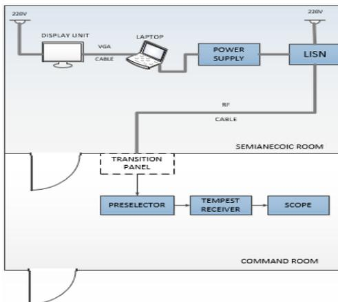
Fig. 4. Test configuration setup – LISN measurements
