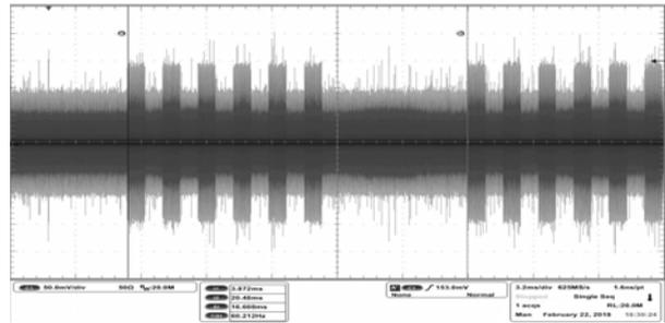
Fig. 6. Video signal - 6 horizontal lines, using MDS-21 clamp and a commercial power cable
