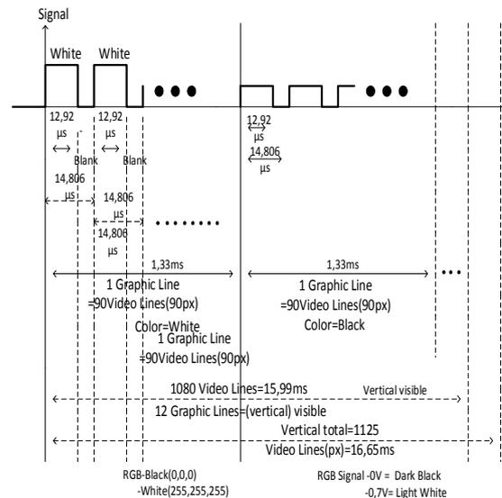
Fig. 2. The structure of the 6 white stripes and 6 black stripes - video resolution of 1920 x 1080 at 60 (Hz) refresh rate
