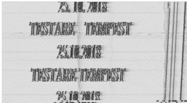
Fig. 9. Video image recovery - 24 font text, commercial power supply
