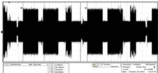
Fig. 7. Video signal - two thick horizontal bars and a thin one, using a LISN and a commercial power supply
