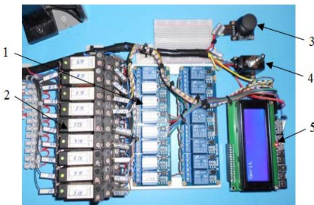
Fig. 6. Command and control system: 1- output relay module; 2- input relay module; 3- joystick; 4- operation mode selection switch; 5- microcontroller development system.
