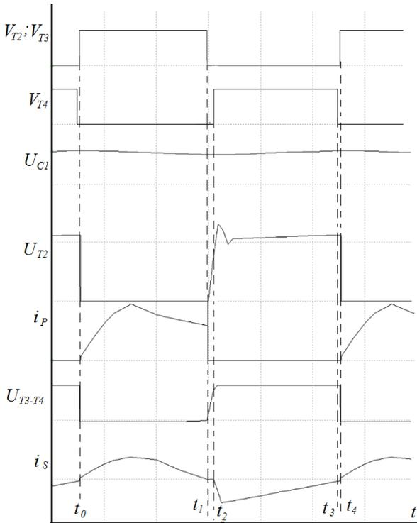
Fig. 5. Diagram of switching processes of transistors of the SST transformer for the zero switching mode (ZCS mode).
