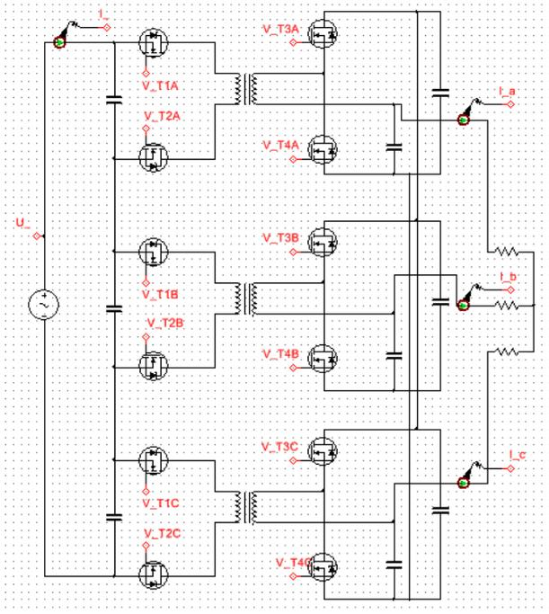
Fig.6. Model for simulating the operation modes of the SST transformer
