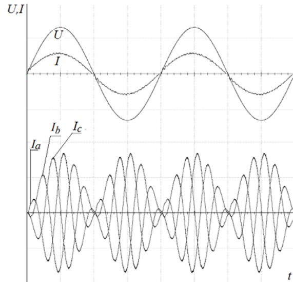
Fig. 11. The input voltage  $U$  and current  $I$  to SST power supply from single phase AC at 50 Hz and the curves of the output phase currents  $I_a$ ,  $I_b$ ,  $I_c$ , which has of the frequency 200 Hz (relative units)
