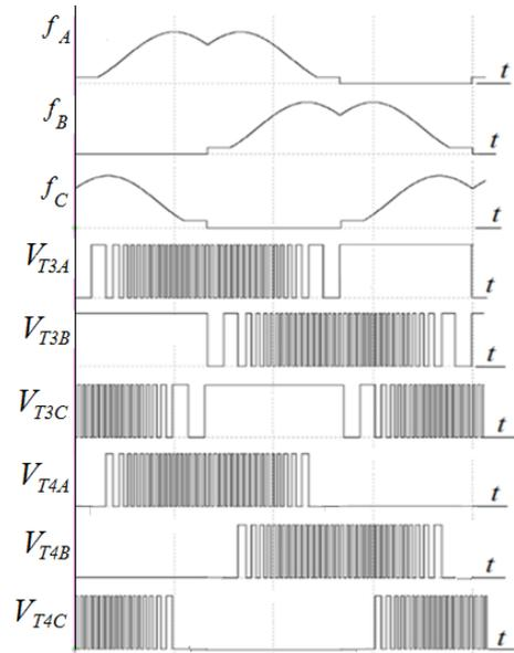
Fig. 4. The law of command pulse generation
