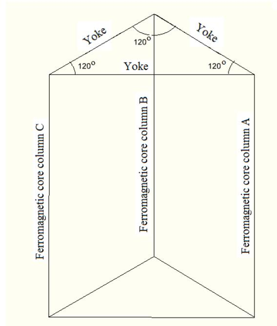
Fig.2. Schematic of the spatial location the columns of the ferromagnetic core of the SST transformer.
