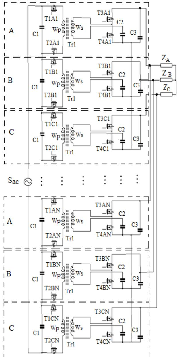
Fig. 1. Equivalent scheme of single-phase/three-phase bidirectional SST.
