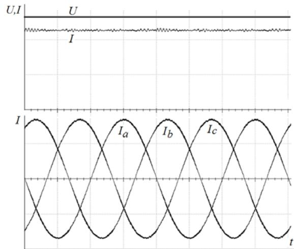
Fig.8. Input voltage  $U$  and current  $I$ , the output phase currents  $I_a, I_b, I_c$  of the SST transformer at the frequency of 50 Hz (relative units)
