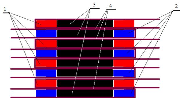
Fig.3. The scheme of placed the coils of the SST transformer phase on the ferromagnetic core column.
