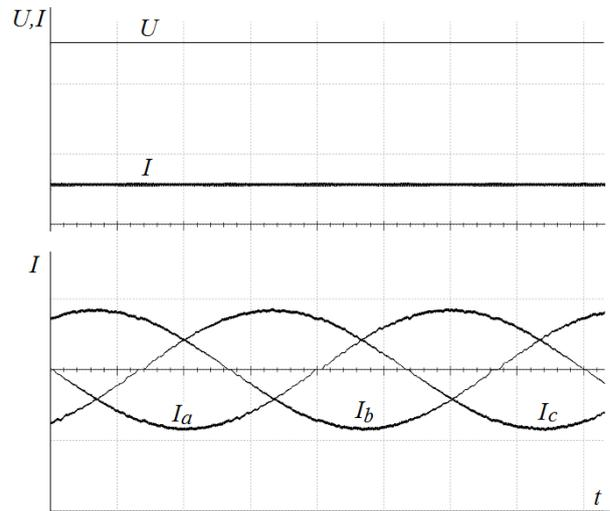
Fig.7. Input voltage  $U$  and current  $I$ , the output phase currents  $I_a, I_b, I_c$  of the SST transformer at the frequency of 25 Hz (relative units)
