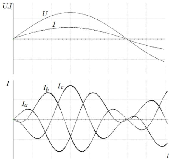
Fig. 9. Input voltage  $U$  and current  $I$  to SST power supply from single phase AC at 16.7 Hz and the curves of the output phase currents  $I_a$ ,  $I_b$ ,  $I_c$ , which has of the frequency 50 Hz (relative units)
