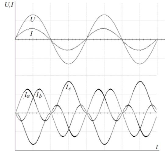
Fig. 10. Input voltage  $U$  and current  $I$  to SST power supply from single phase AC at 50 Hz and the curves of the output phase currents  $I_a$ ,  $I_b$ ,  $I_c$ , which has of the frequency 50 Hz (relative units)
