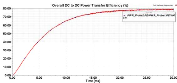
Fig. 13. Overall DC-to-DC power transfer efficiency.
