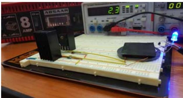
Fig. 7. The measured voltage in the receiver inductor for the case in which both inductors are situated on ferrite.
