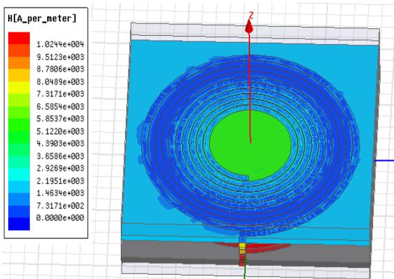
c) Magnetic field intensity for a distance of 1 mm
