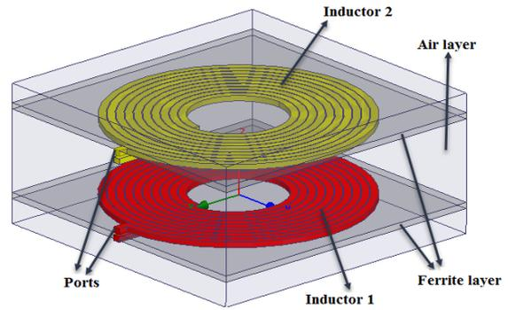
c) Spiral inductor considering the emitter and receiver inductors on a ferrite layer
