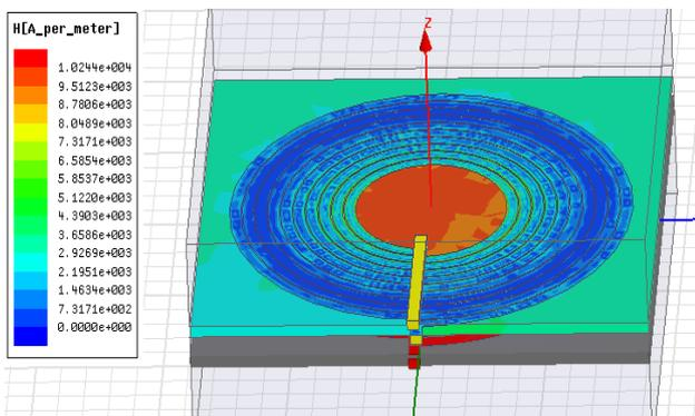
d) Magnetic field intensity for a distance of 0.05 mm
