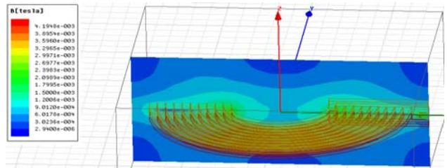
Fig. 10. Magnetic induction for different distances between the two spiral inductors considered.
