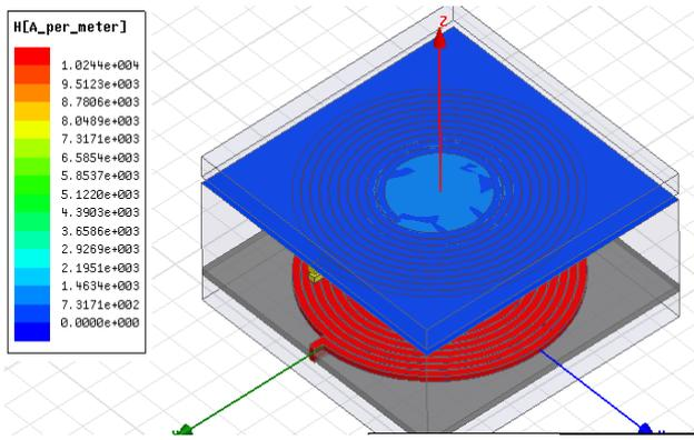
a) Magnetic field intensity for a distance of 5 mm
