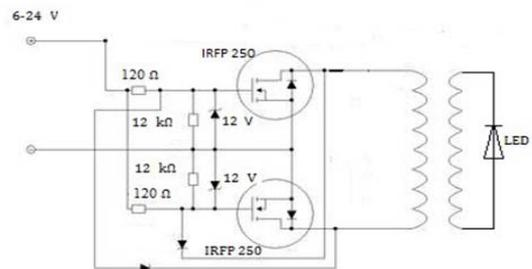
Fig. 4. Electrical scheme of the first power system.
