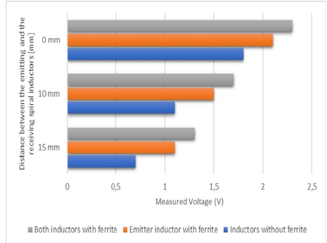
Fig. 8. The measured voltage in the receiver inductor for the three cases considered and at different distances between the inductors.
