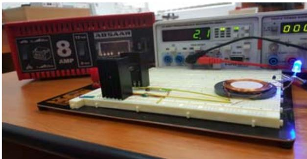
Fig. 6. The measured voltage in the receiver inductor for the case in which the emitter inductor, is situated on the ferrite.
