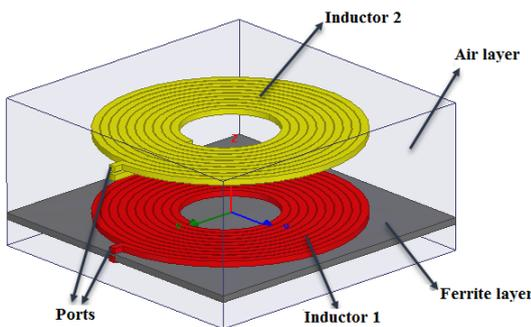
b) Spiral inductor considering the emitter inductor on a ferrite layer
