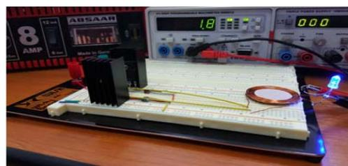
Fig. 5. The measured voltage in the receiver of the wireless system without ferrite.
