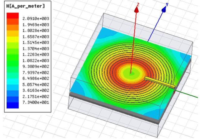
Fig. 11. Magnetic field intensity for different distances between the two spiral inductors considered and the emitter on a ferrite layer.
