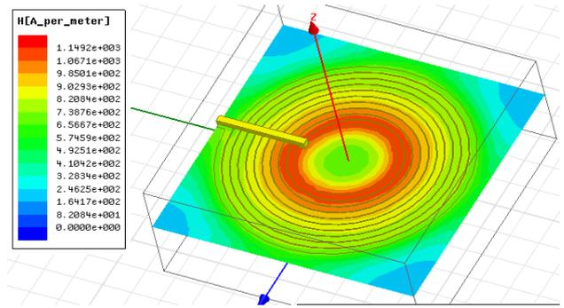
Fig. 9. Magnetic field intensity for different distances between the two spiral inductors considered.
