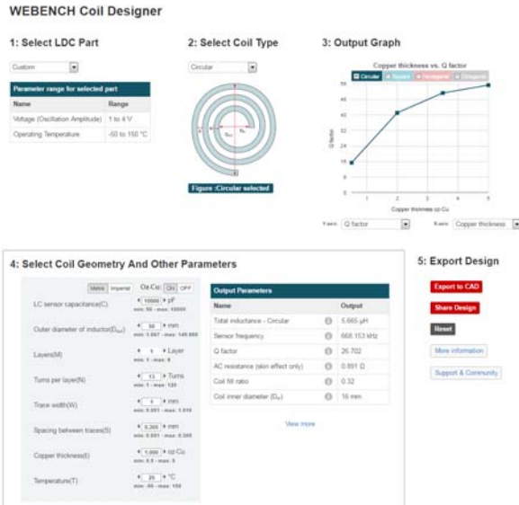
Fig. 1. WEBENCH overview showing the main components (and steps) of this tool: 1. Select LDC Part, 2. Select Coil Type, 3. Output Graph, 4. Select Coil Geometry And Other Parameters, 5. Export Design.
