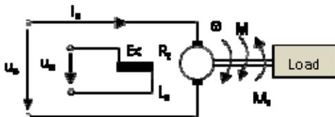
Fig.4 An DC motor drive structure
