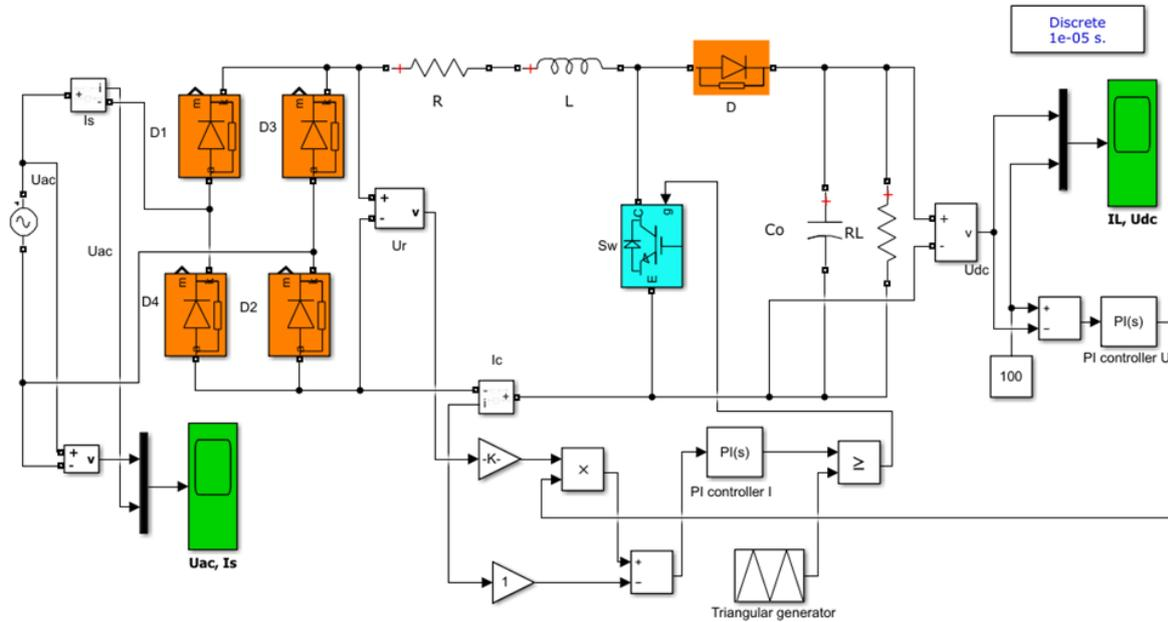
Fig. 14. The Matlab / Simulink model of the circuit shown in Fig. 5. The average current control method avoids the complications of the peak current control method by using a high gain integrative amplifier in the current feedback loop [3].
