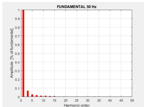
Fig. 16. Harmonic spectrum of the current in Fig.15.
