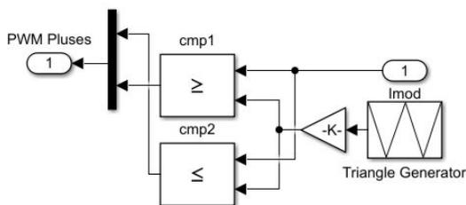
Fig. 8. PWM modulator structure.
