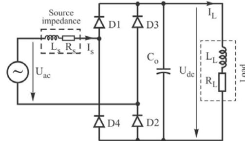
Fig. 1. Schematic of a single-phase uncontrolled bridge rectifier.
