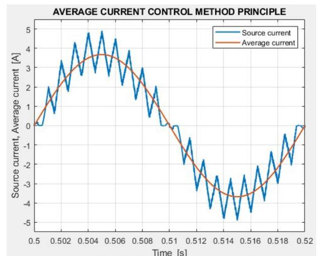
Fig. 13. Waveforms for control by average current value.
