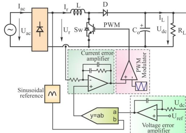
Fig. 12. Block diagram of the PFC boost converter controlled by the average current value ([3]).
