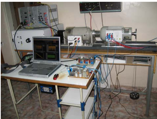
Fig.4. Experimental test bench with the application of the mechanical brake: a. schematic diagram; b. general view
