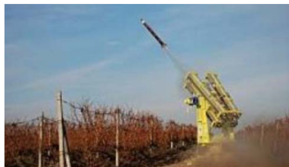
Fig. 1. The missiles launch ramp used by the Romanian Anti-Hail System
