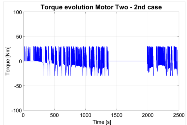
Fig. 17. Torque on the smallest motor in the second case.
