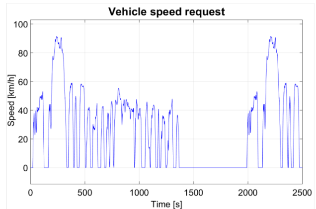
Fig. 4. Speed request during the testing cycle (FTP75).
