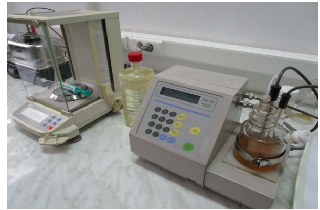
Fig. 2. The image of the Karl-Fisher coulometric titrator model CA-21 used in the experimental results.
