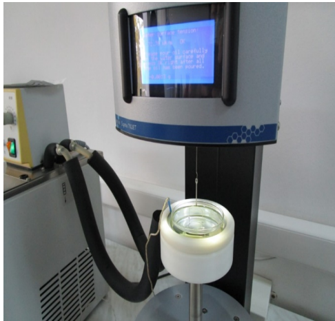
Fig. 3. The image of the tensiometer type KSV Sigma 702ET used in experiments.
