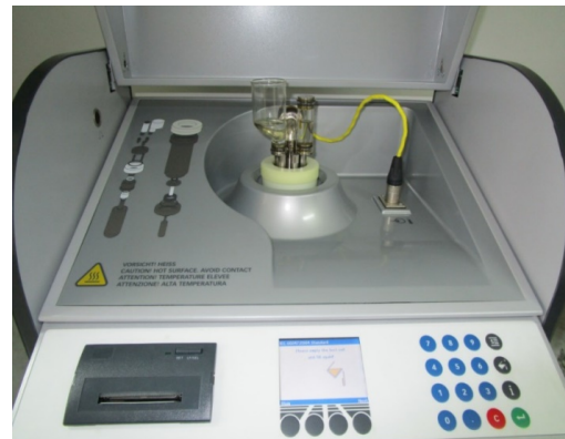
Fig.8. The image of the BAUR DTLC tester.
