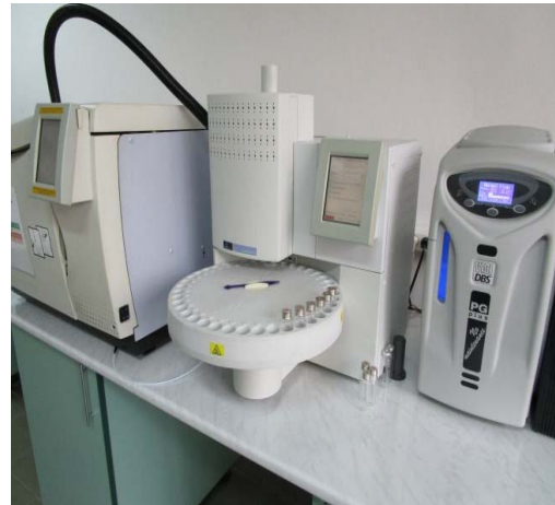
Fig. 4. The image of the chromatograph type CLARUS 600 that was used in tests
