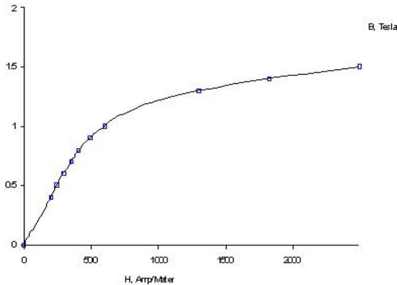
Fig. 2. Non-linear characteristic  $B(H)$  of magnetic material
