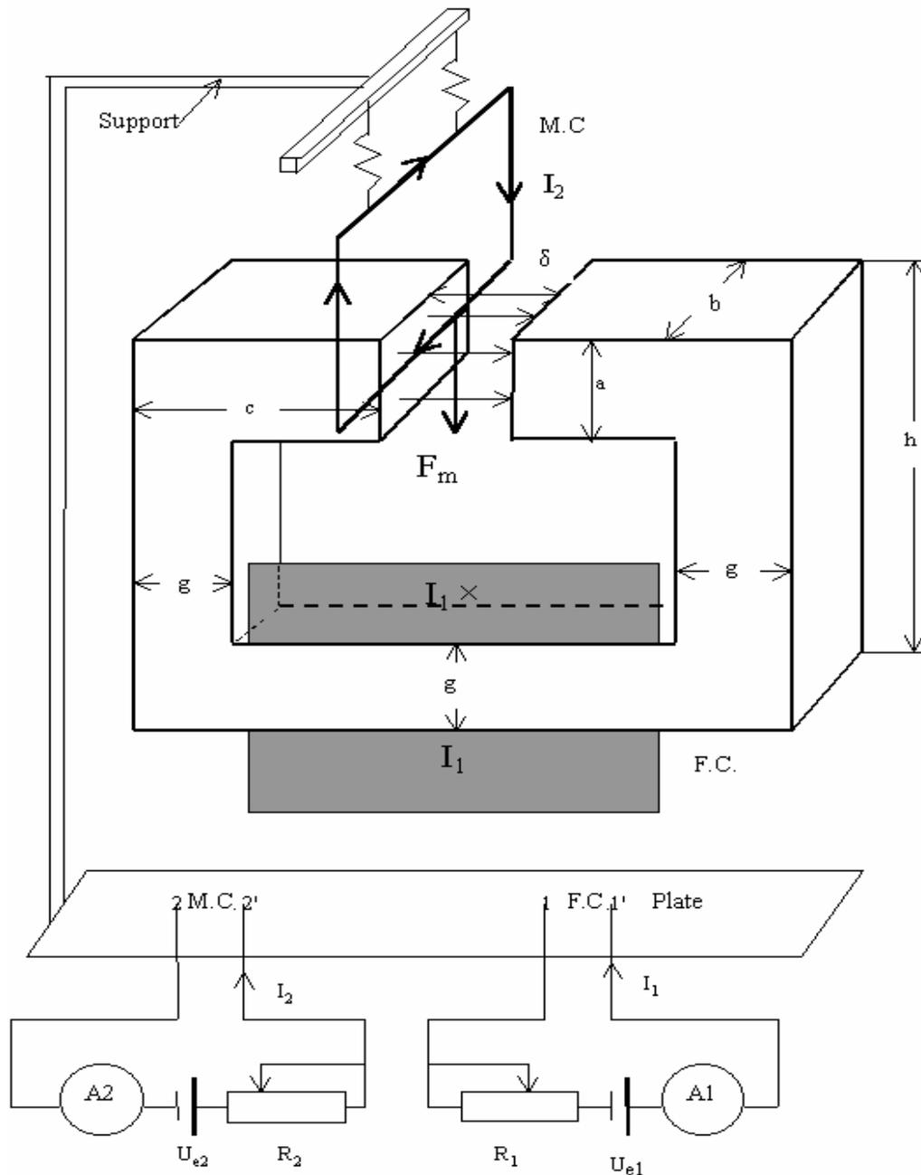
Fig. 1. Experimental schematic: M.C. - mobile coil, F.C. - fixed coil,  $F_m$  - magnetic force,  $B = B(I_1)$  - magnetic flux density
