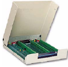
Figure 7: Carte d'acquisition analogique
