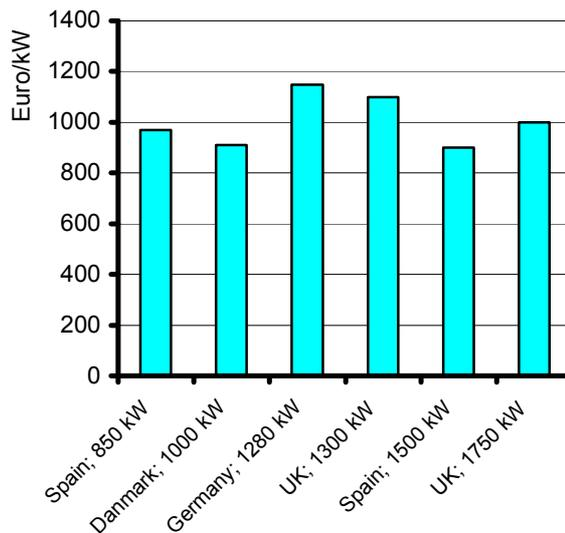
Figure 1: Total investment cost for different turbine sizes and countries of installation
